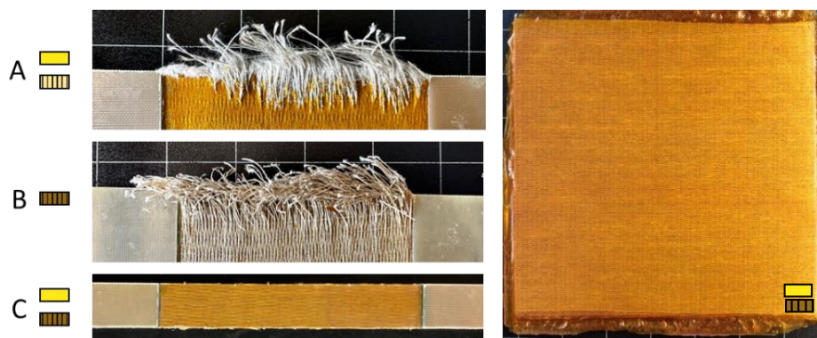
Figure 5: Tensile test specimens manufactured by processes A-C (left); composite plate made by process C (right).
