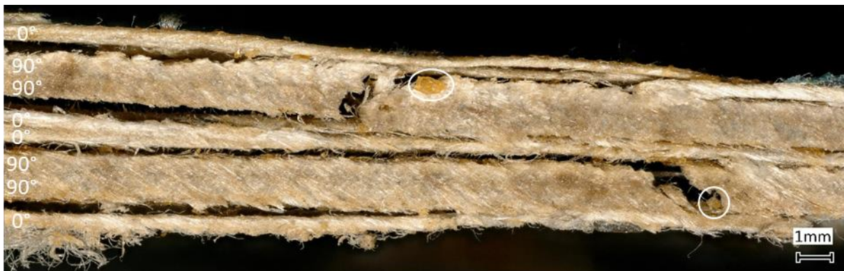
Figure 8: Fracture pattern of a cross-ply specimen after tensile test. Ellipses indicate gelled particles.
