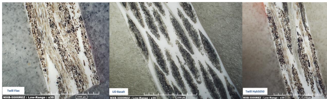
Figure 7: Microscopic view of basalt/PA11 UD composite, flax/PA11 twill composite and hybrid5050/PA11 twill composite
