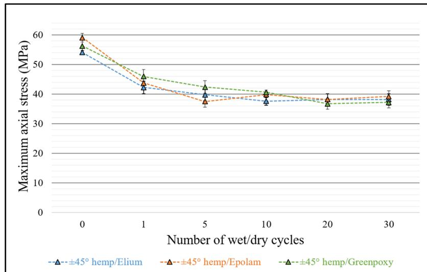
Figure 3: Maximum axial stress of  $\pm 45^\circ$  hemp-reinforced composites versus the number of wet/dry cycles (0 means “Ambient storage”).
