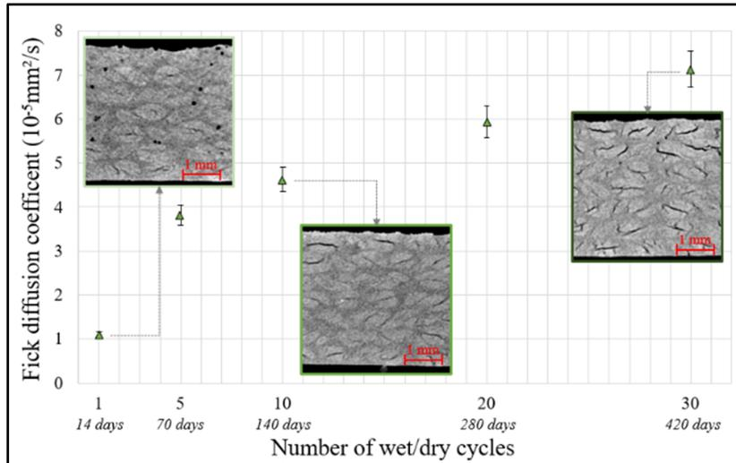
Figure 2: Fick diffusion coefficient evolution for hemp/Greenpoxy  $[\pm 45^\circ]_7$  samples and related micro-CT images after 1, 10 and 30 wet/dry cycles.
