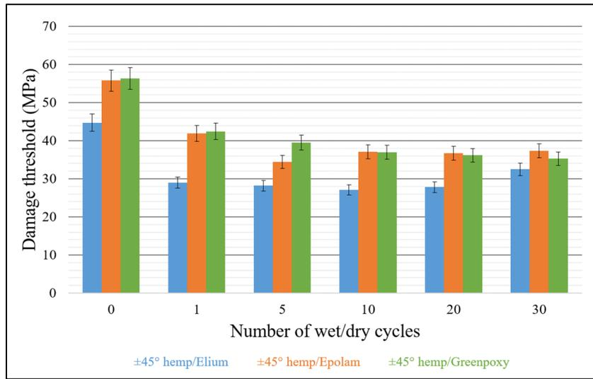
Figure 4: Applied stress values to reach 5% of the total AE cumulated energy during tensile testing of ±45° hemp-reinforced composites versus the number of wet/dry cycles (0 means “Ambient storage”).
