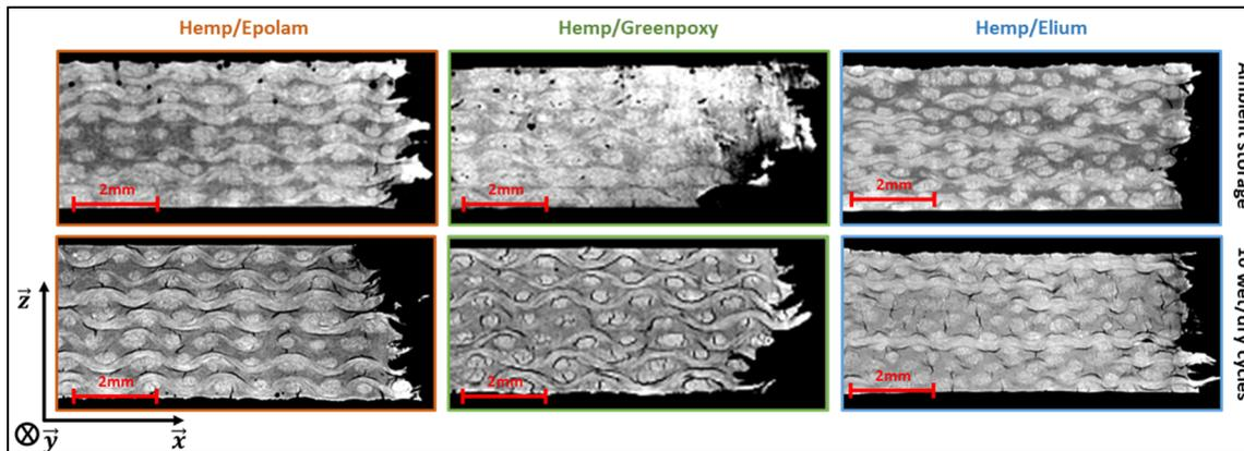
Figure 6: Micro-CT images after tensile testing for the three different biocomposites (orientation  $0^\circ/90^\circ$ ) after ambient storage and ten wet/dry cycles.
