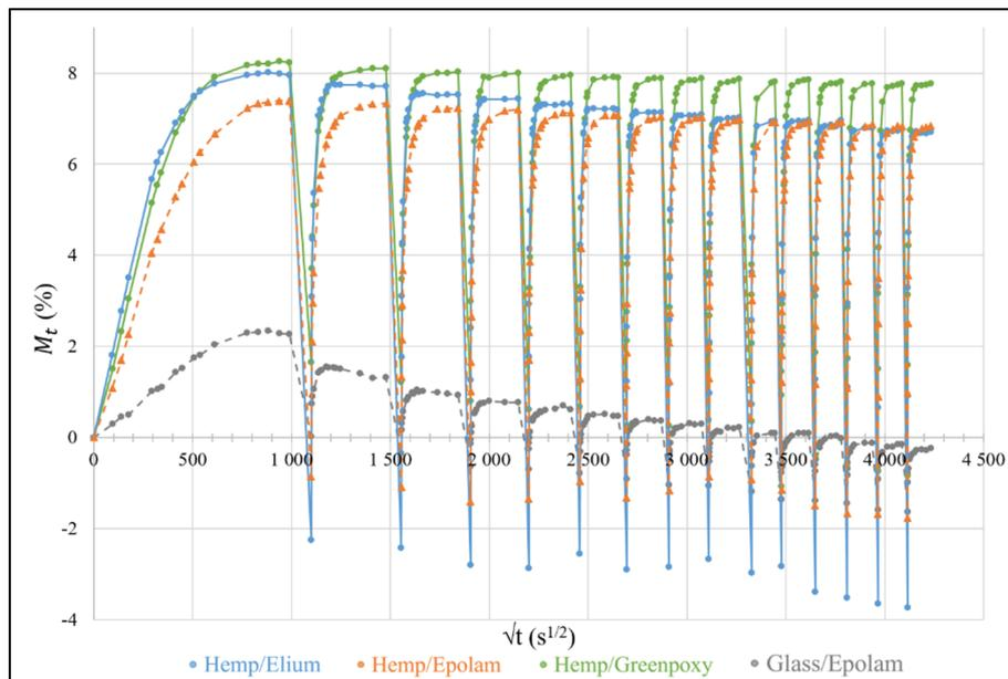
Figure 1: Weight variations during fifteen wet/dry cycles for all the studied materials.
