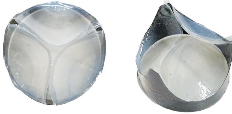
Figure 1: Top (left) and side (right) view of heart valve implants with carbon fiber composite stents
