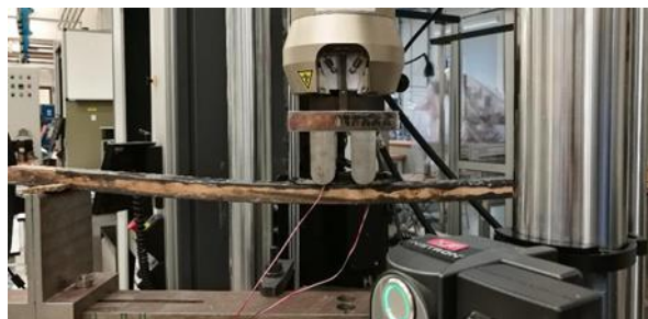
Figure 4: Experimental setup for the 4-point flexural test with the sandwich beam.
