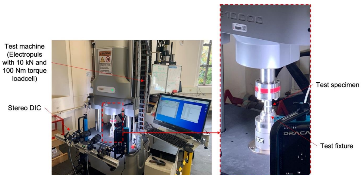
Figure 3: The test setup to conduct pure shear and compression-shear tests.
