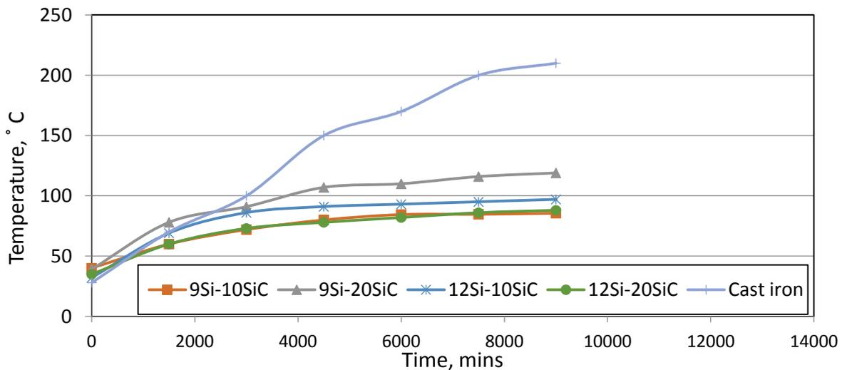
Fig. 10 Temperature behavior of Al-Si composite brake rotors and commercial cast iron brake rotor at speed of 5 m/s and load of 23.06 N
