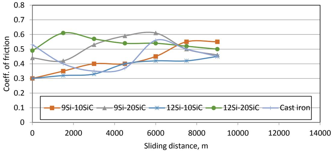
Fig. 6 Coefficient of friction of composite brake rotors produced and commercial cast iron brake rotor at load of 23.06 N and speed of 5m/s
