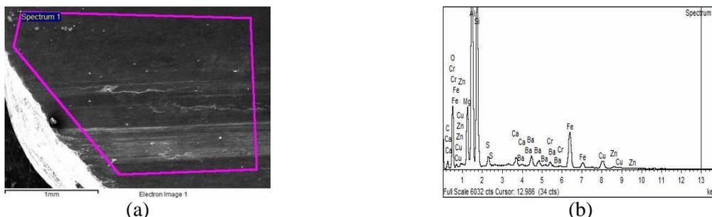
Fig.4.2 Worn surface of brake rotor made of Al12Si + 10%SiC at load of 35.6 N and speed of 7m/s , a) low magnification of worn surface of Al12Si+10%SiC, b) EDX for Al12Si+10%SiC
