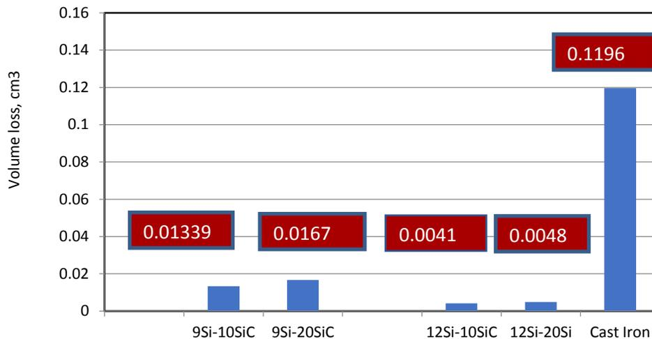
Fig. 5 Volume loss of Al-Si composite Brake rotors and commercial cast iron brake rotor at speed of 7m/s and load of 35.6 N
