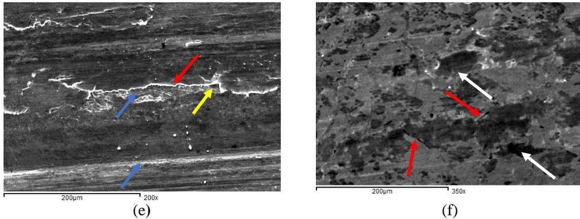
Fig. 14 Worn surface of brake rotor made of Al12Si + 10%SiC compared and commercial one made of cast iron at load of 35.6 N and speed of 7m/s, a) low magnification of worn surface of Al12Si+10%SiC, b) EDX for Al12Si+10%SiC, c) low magnification of worn surface of cast iron, d) EDX of cast iron worn surface, e) higher magnification of worn surface of Al12Si+10%SiC, f) higher magnification of worn surface of cast iron
