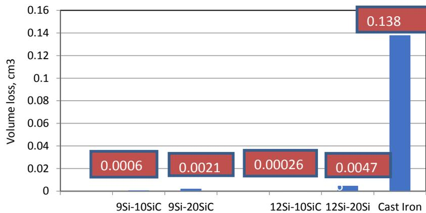
Fig. 4 Volume loss of Al-Si composite brake rotors and commercial cast iron brake rotor at speed of 5 m/s and load of 35.6 N
