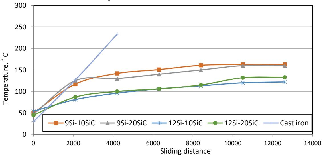
Fig. 13 Temperature behavior of Al-Si composite brake rotors and commercial cast iron brake rotor at speed of 7 m/s and load of 35.6 N
