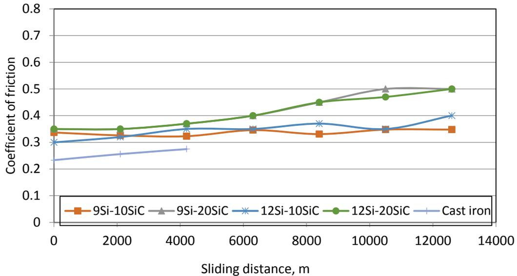
Fig. 9 Coefficient of friction of composite brake rotors produced and commercial cast iron brake rotor at speed of 7m/s and load of 35.6 N
