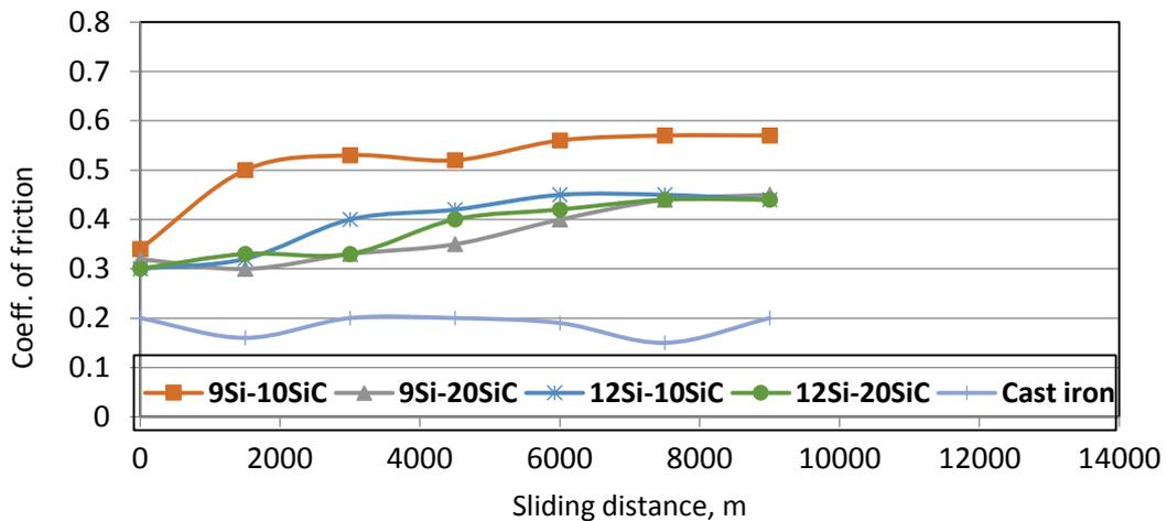
Fig. 8 Coefficient of friction of composite brake rotors produced and commercial cast iron brake rotor at speed of 5m/s and load of 35.6 N
