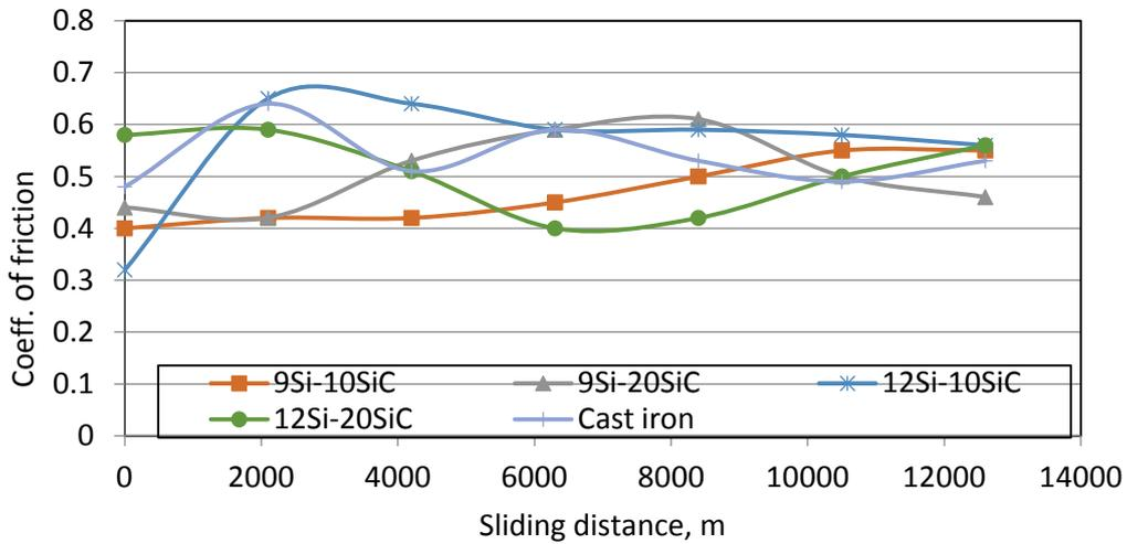
Fig. 7 Coefficient of friction of composite brake rotors produced and commercial cast iron brake rotor at load of 23.06 N and speed of 7m/s
