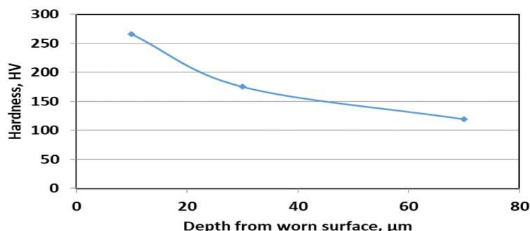
Fig.4.3 Microhardness of mechanically mixed layer
