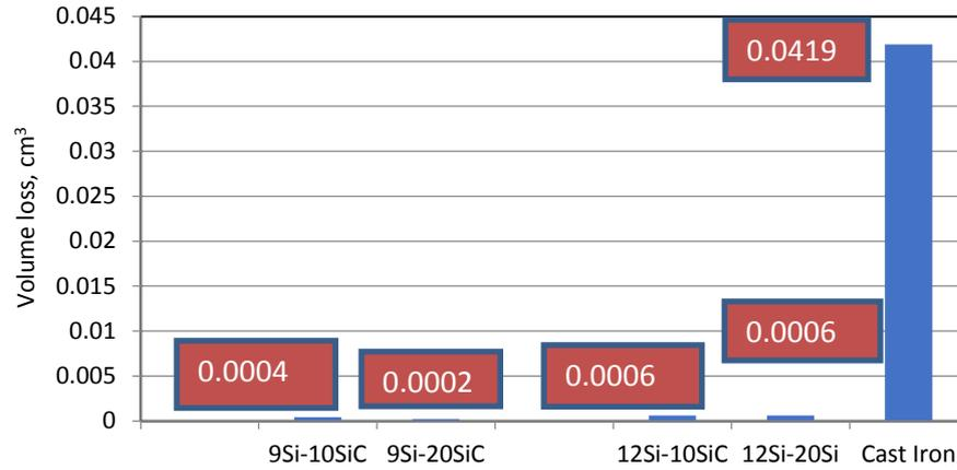
Fig. 2 Volume loss of Al-Si composite brake rotors and commercial cast iron brake rotor at speed of 5 m/s and load of 23.06 N
