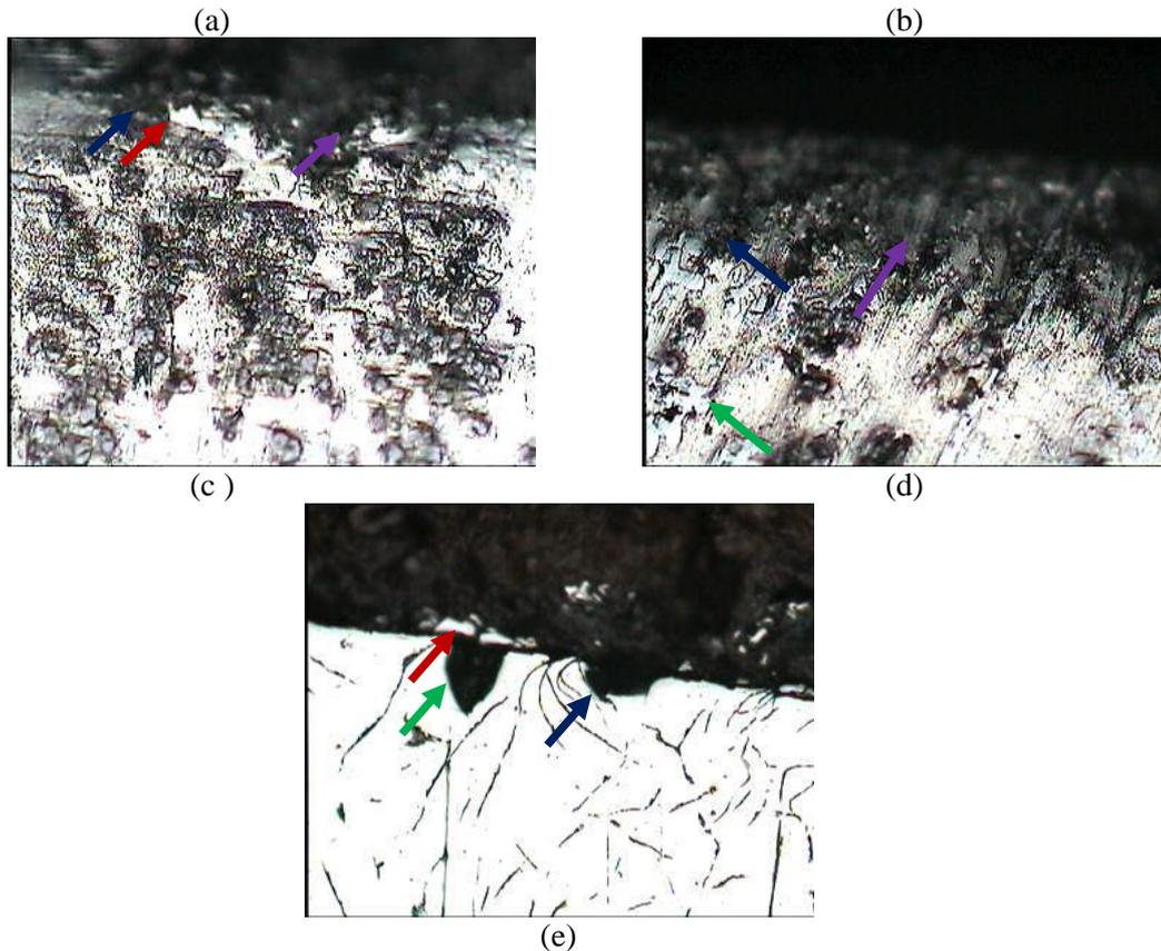
Fig.15 Subsurface of worn surface of produced composite brake rotors and commercial cast iron one, (a) 9Si-10SiC, (b) 9Si-20SiC, (c) 12Si-10SiC, (d) 12Si-20SiC, (e) cast iron
