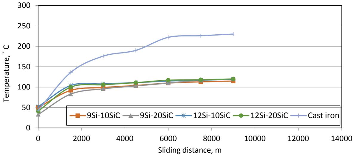
Fig. 12 Temperature behavior of Al-Si composite brake rotors and commercial cast iron brake rotor at speed of 5 m/s and load of 35.6 N
