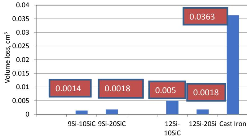
Fig. 3 Volume loss of Al-Si composite brake rotors and commercial cast iron brake rotor at speed of 7 m/s and load of 23.06 N
