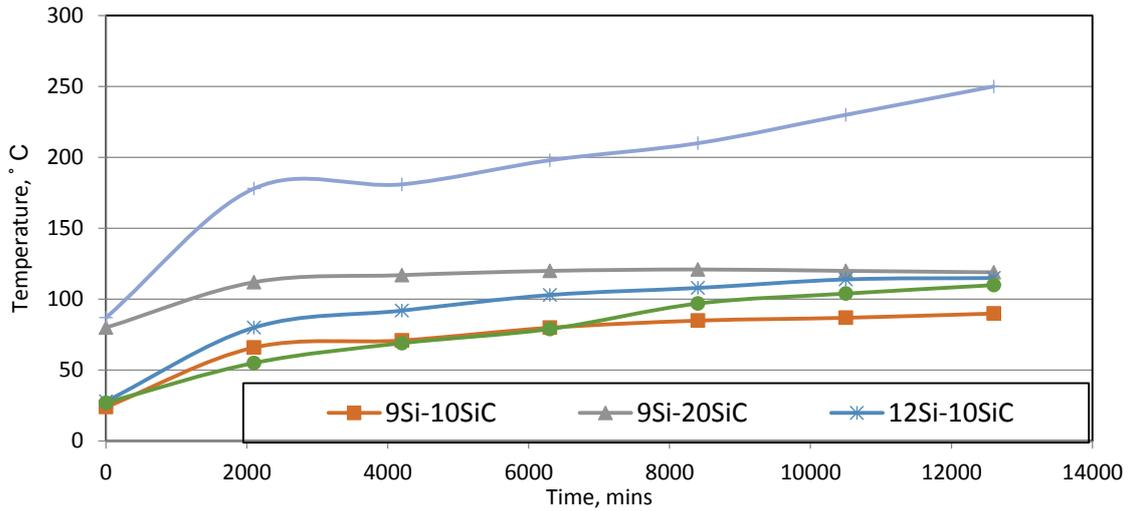
Fig. 11 Temperature behavior of Al-Si composite brake rotors and commercial cast iron brake rotor at speed of 7 m/s and load of 23.06 N
