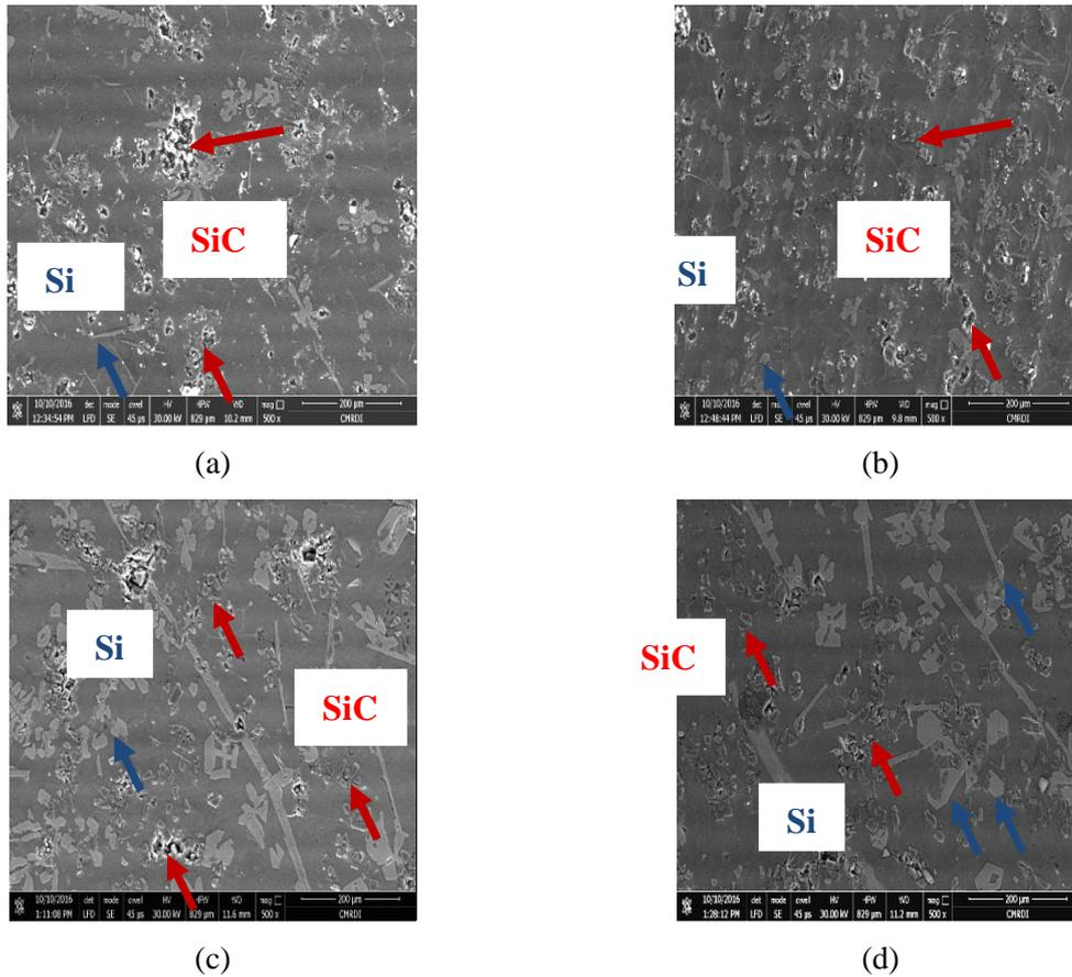
Fig.1 (a-d) FEM microstructure of the composite brake rotors after heat treatment, (a) Al-9Si+10SiC, (b) Al-9Si+20SiC, (c) Al-12Si+10SiC, (d) Al-12Si+20SiC
