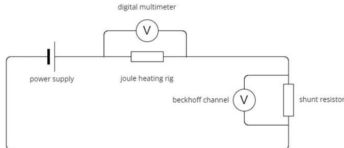
Figure 2 Electric circuit for static joule heating testing
