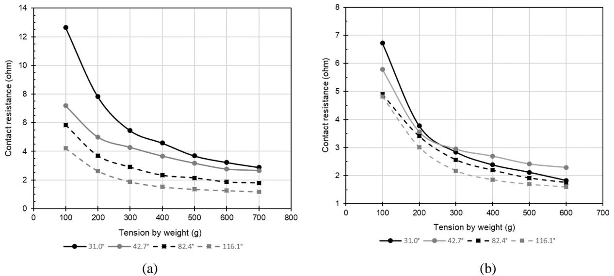
Figure 5 Total contact resistance results (a) without current (b) with current passing in the circuit
