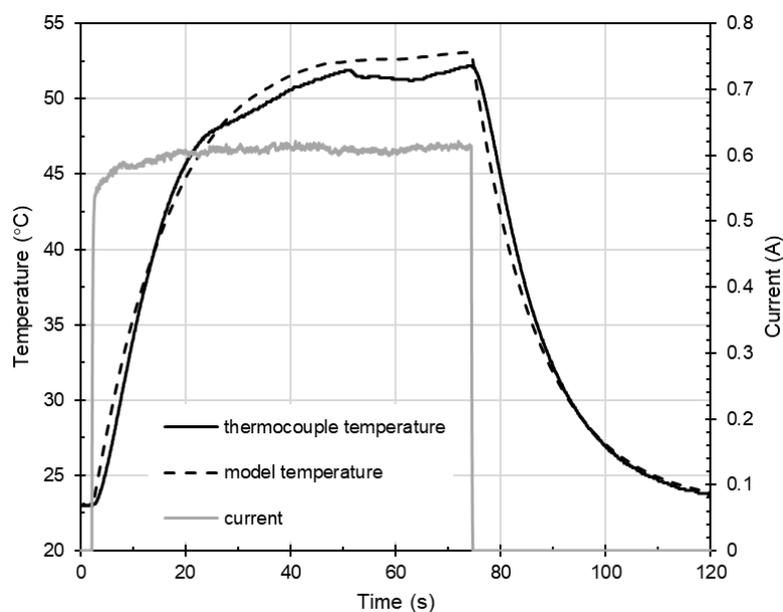
Figure 9 Heating and cooling curve of carbon fibre tape under a step current input
