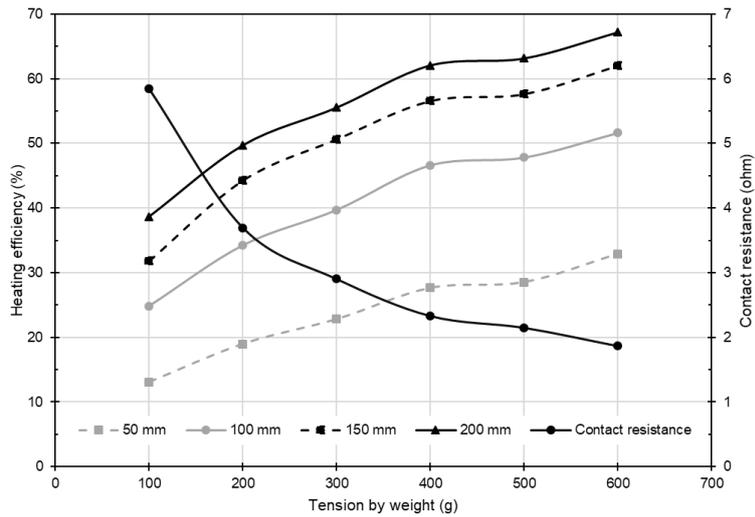
Figure 6 Joule heating efficiency results at contact angle of 82.4°
