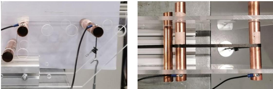
Figure 1 Joule heating rig: front view and top view
