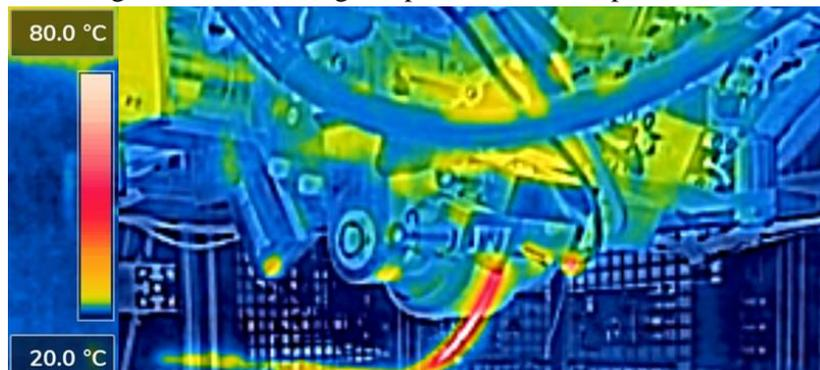
Figure 4 Thermal camera temperature measurement for dynamic joule heating test in the ADFP head
