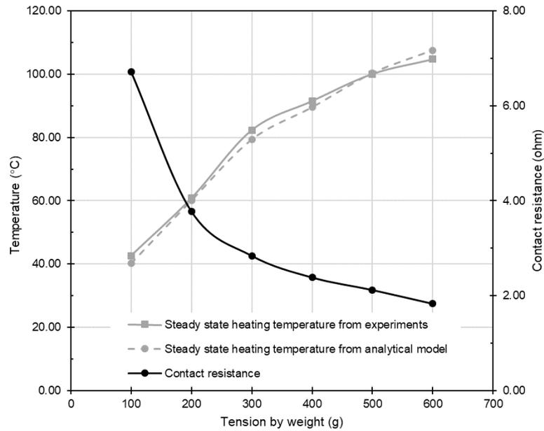
Figure 7 Static joule heating results for 50 mm length with 31.0° contact angle under a constant voltage supply
