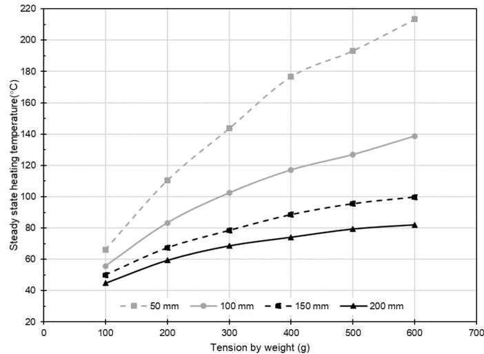
Figure 8 Analytical results of steady state heating temperature for 31.0° contact angle with a constant voltage of 5 V
