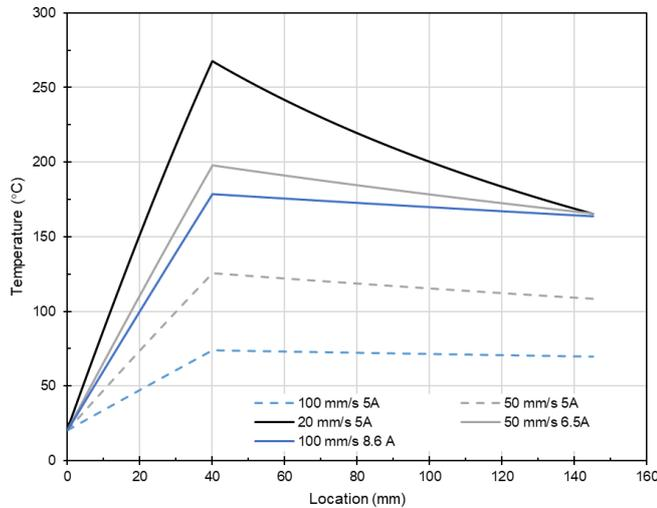
Figure 11 Model calculated temperature distribution in the ADFP head from heating region to the nip point (the right end is the nip point)
