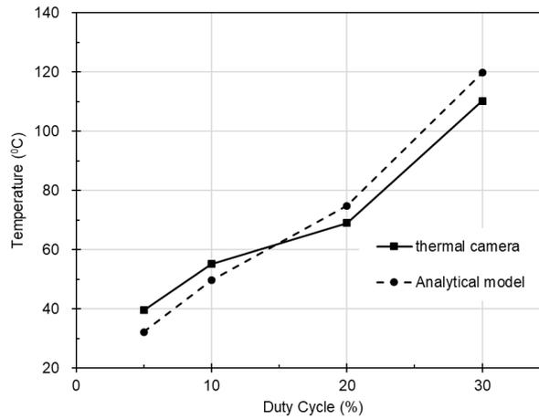
Figure 10 Nip point temperature from dynamic joule heating with 100 mm/s feeding velocity
