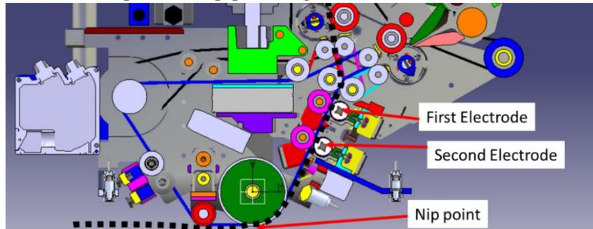
Figure 3 Joule heating setup in the ADFP deposition head
