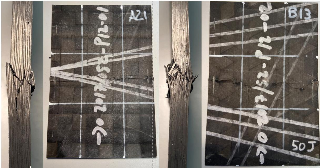
Figure. 7. Crack path and cross-section of fracture plane in crossply and quasi-isotropic CAI specimens impacted at 50 J.
