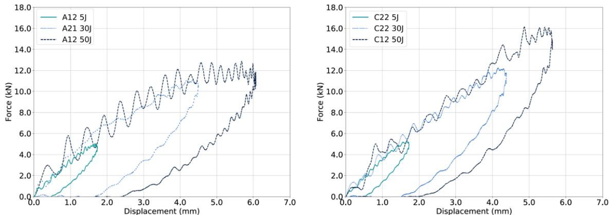
Figure 4. Representative force vs displacement curves at different energy levels for (a) AP-PLY crossply panel and (b) AP-PLY triaxial panel.
