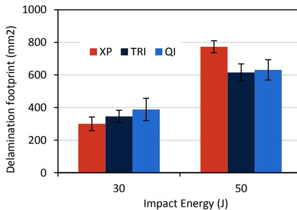
Figure 6. Delamination as function of the impact energy.
