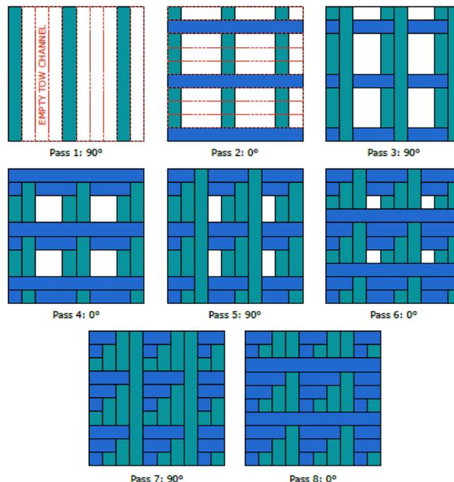
Figure 1. Schematic illustrating the layup process of a cross-ply AP-PLY laminate tape spacing of 3.
