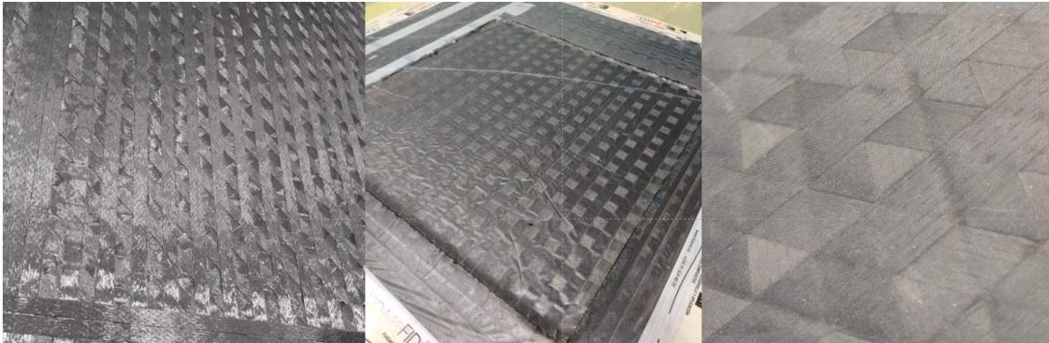
Figure 2. AP-PLY manufacturing process. (a) Dry fibre preform created by AFP, (b) resin transfer moulding and (c) final surface quality.
