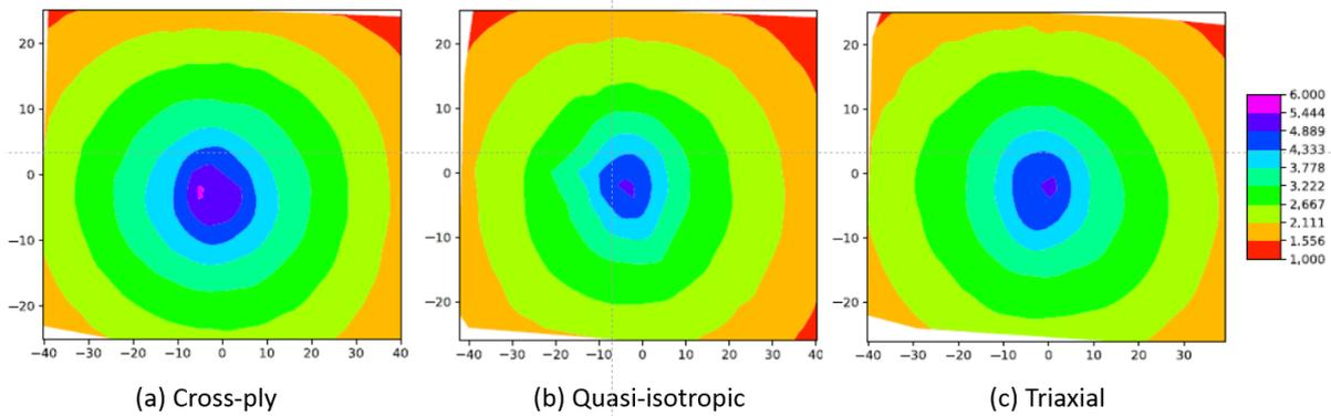
Figure 5. Maximum deflection of the panels at the peak force. Deflection in mm.
