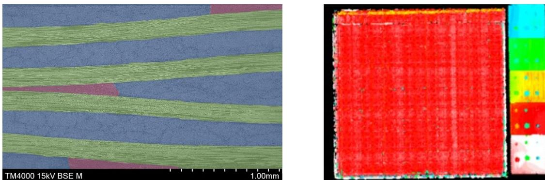
Figure 3. (a) SEM micrographs showing the characteristic tow undulations in green, the perpendicular tows in blue and the resin pockets in red. (b) Preliminary C-Scan measurements and comparison against baseline plates.
