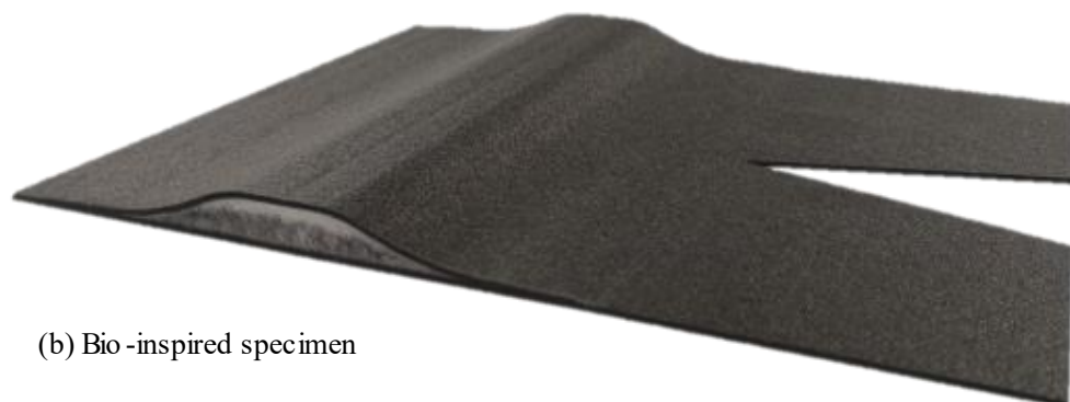
Figure 8: Stiffened panel test specimens following water-jet cutting.
