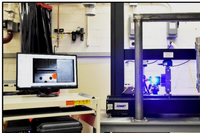
Figure 2: (a) 5-pin compact tension sample geometry consisting of 12 layers of woven fabric, and (b) compact tension test setup used for fracture testing monitored with DIC camera.
