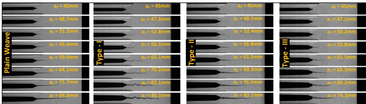
Figure 6: Crack path for the propagation for composites with weave patterns: (a) Plain weave, (b) Type-I, (c) Type-II, and (d) Type-III.
