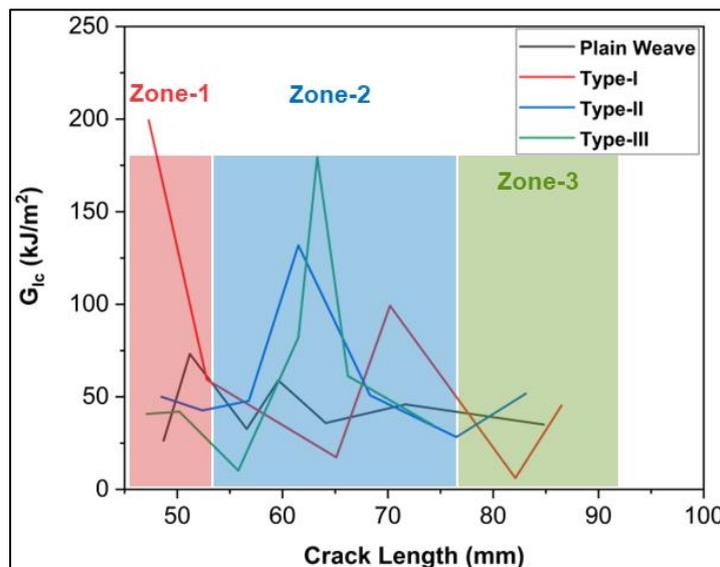
Figure 7: Fracture toughness ( $G_{Ic}$ ) vs crack length for all four weave patterns showing higher variations for Type-I, Type-II, and Type-III composites due to heterogenous weave architectures.
