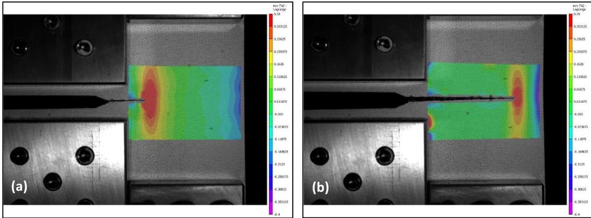
Figure 4: (a) Fracture process zone (FPZ) at the crack front in Zone-2 (b) Fracture process zone (FPZ) at the crack front in Zone-3 showing the interacting stress concentrations.
