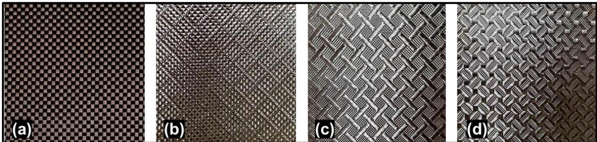
Figure 1: Weave patterns tested: (a) Plain weave (*Type 0*), (b) M-Boss weave (*Type I*), (c) Diamond plate weave (*Type II*), and (d) Roswell weave (*Type III*).
