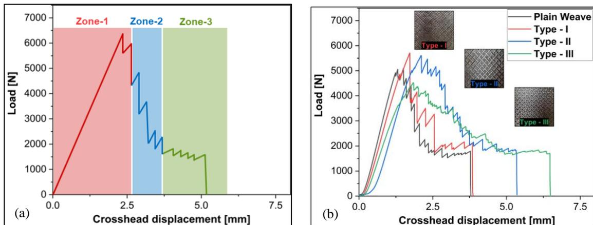
Figure 3: (a) Schematic of the Load-crosshead displacement curve for woven composites and (b) Representative load-crosshead displacement curves for composites with four weave patterns.
