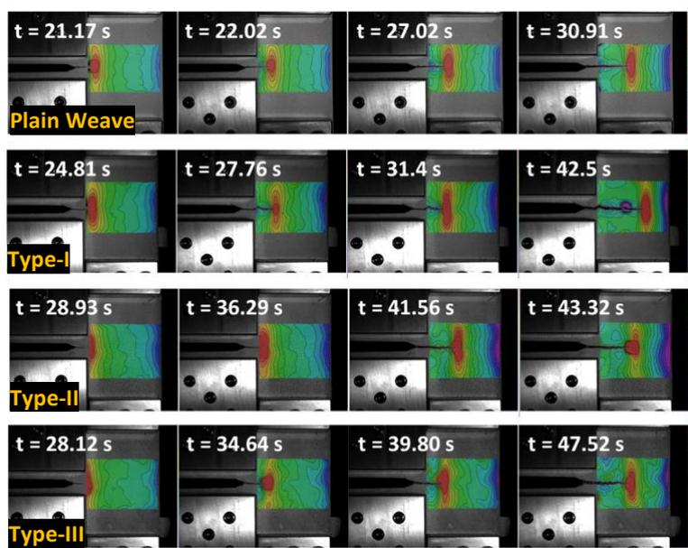
Figure 5: (a) Fracture process zone (FPZ) at the crack front for all weave patterns with a strain range from -0.4% to 0.4%.
