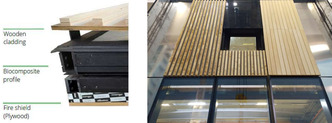
Figure 4. Images of the bio-based profile and the façade fire test (Source: Focchi Group).
