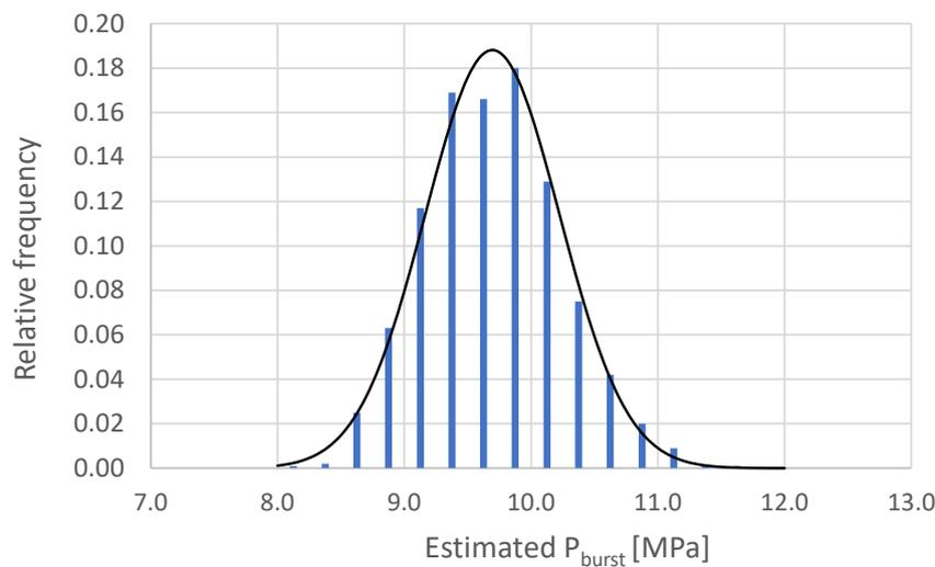
Figure 3: Probabilistic failure response of a COPV to material uncertainty – Histogram of estimated burst pressure.
