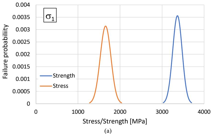
Figure 7: Stress-strength interference on local orientation: (a) Longitudinal normal stress-strength; (b) Transverse normal stress-strength; (c) In-plane shear stress-strength.
