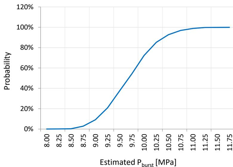
Figure 4: Probabilistic failure response of a COPV to material uncertainty – CDF of estimated burst pressure.
