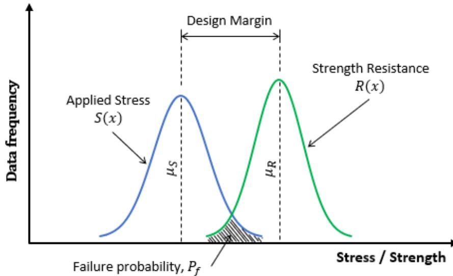
Figure 1: Stress-Strength analysis for reliability: Graphical representation of failure concept.
