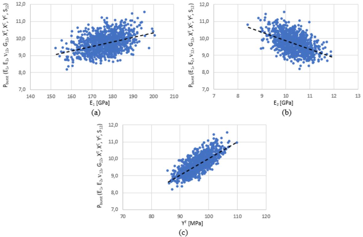
Figure 5: Distribution of estimated burst pressure with respect to: (a) Longitudinal modulus; (b) Transverse modulus; (c) Transverse tensile strength.
