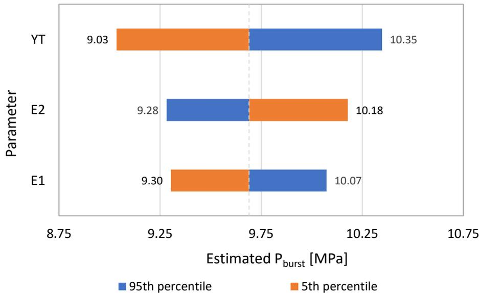
Figure 6: Sensitivity of burst pressure to random input material properties
