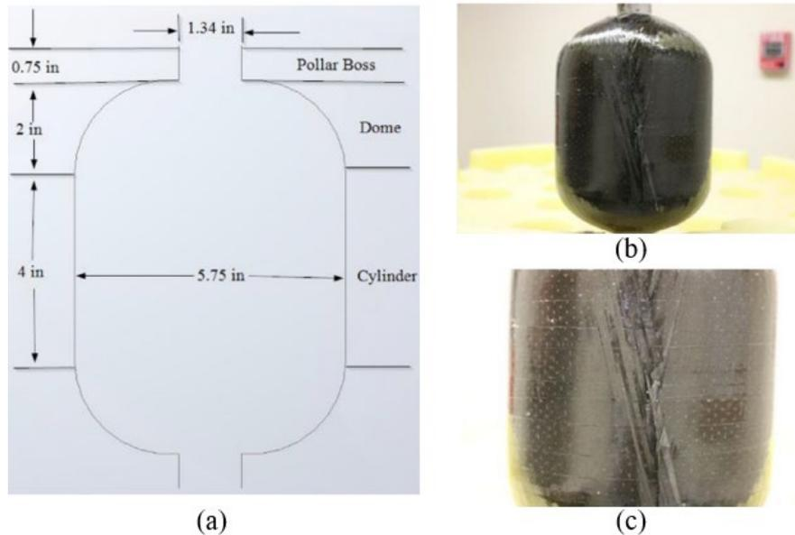
Figure 2: (a) COPV geometry; (b - c) Photographs of failed specimens [6].
