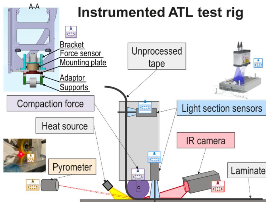
Figure 1 Instrumented ATL test-rig used
