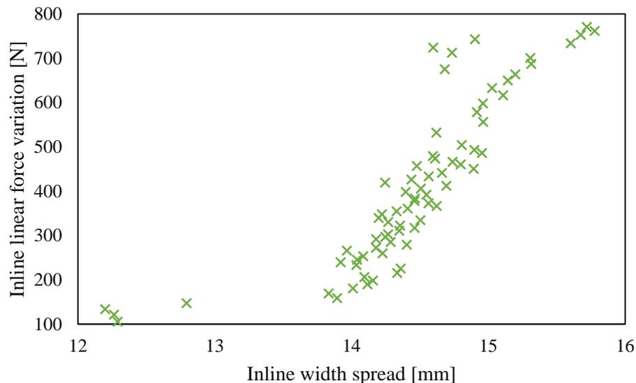
Figure 2 Inline width spread as a result of linearly varying consolidation force
