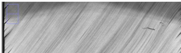
Figure 3 Crack shown in centre of the stacking sequence  $[\pm 45]_{3s}$
