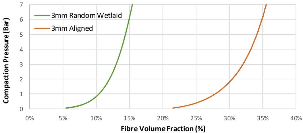
Figure 4 Dry fibre intermediate materials compaction test results.
