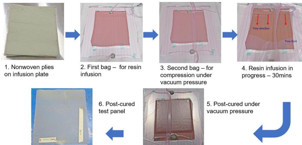
Figure 3. A flow chart of the vacuum infusion process
