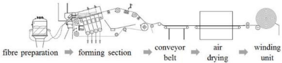
Figure 2. A schematic representation of the wet-laid process.[6]
