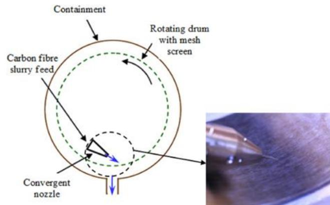
Figure 1. A schematic representation of the hydrodynamic alignment process [5].
