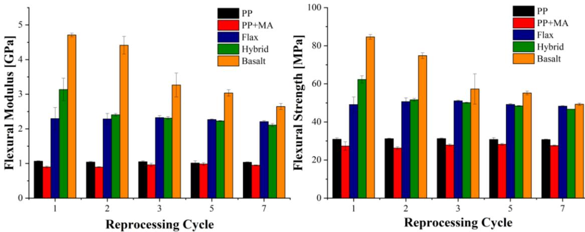
Figure 4: Flexural modulus and strength of the different configurations at the different reprocessing cycles
