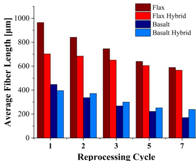
Figure 1: Average fibre length of flax, basalt and hybrids as a function of the number of reprocessing cycles
