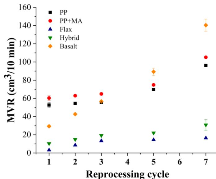
Figure 2: MVR index for formulations under study as a function of the number of reprocessing cycles
