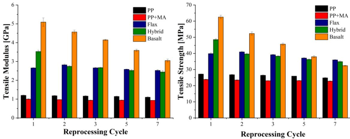
Figure 3: Tensile modulus and strength of the different configurations at the different reprocessing cycles
