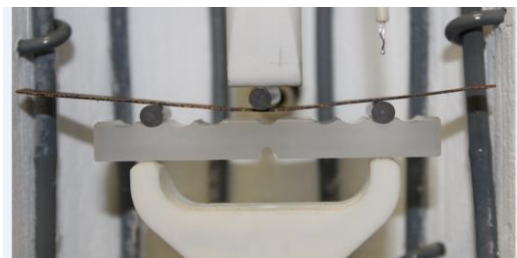
Fig. 3: Flexible Bending Support with Cardanic Piston inside the high temperature furnace
