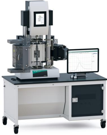
Fig. 1: HT EPLEXOR 500N with standard furnace (-160 °C – 500 °C), right and for high temperature a furnace (RT-1500 °C) for alternative operation (left)
