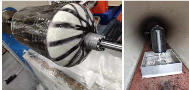
Figure 1: Filament winding on paraffin mandrel and autoclave curing
