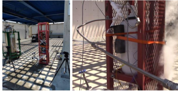
Figure 6: (a) Cryogenic testing setup, (b) Cryogenic Filling
