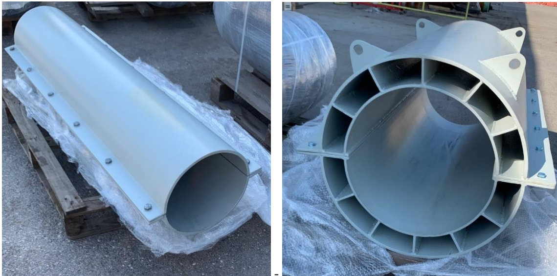
Figure 4: Protection tool inner shell and outer shell
