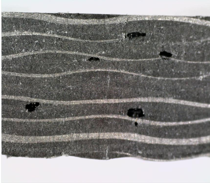
Figure 4: Microscope image of void defects within laminate.
