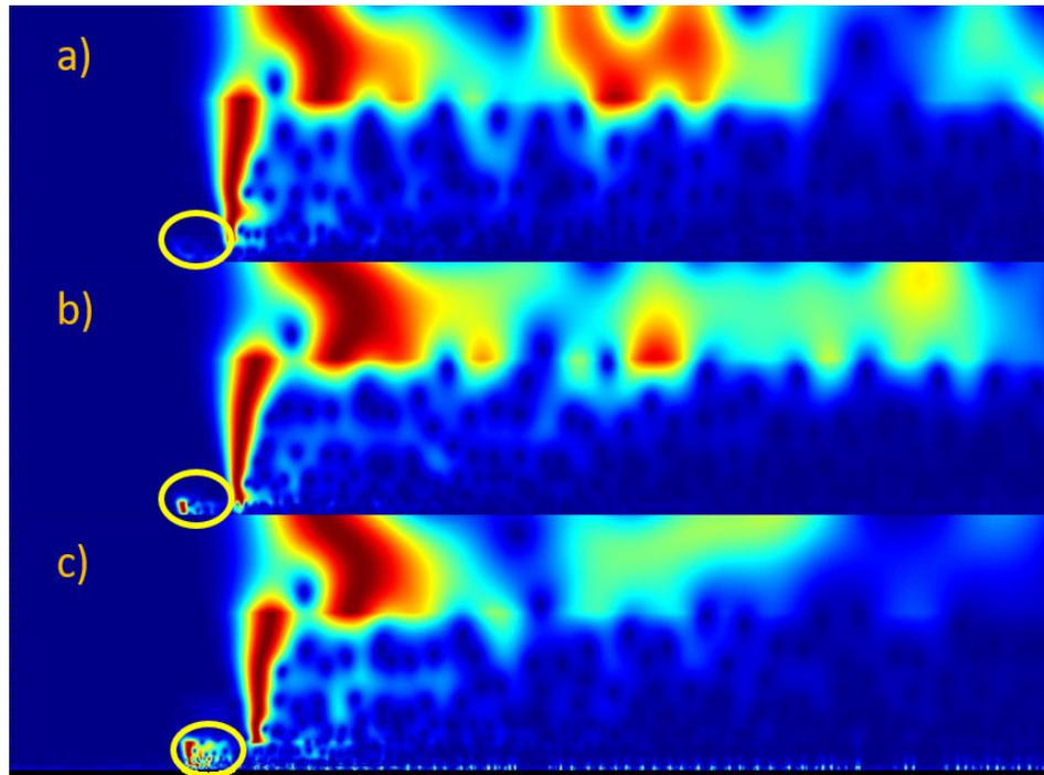
Figure 5: Scalograms for A) Resin Starved, B) Normal Saturation and C) Resin Rich Laminates.
