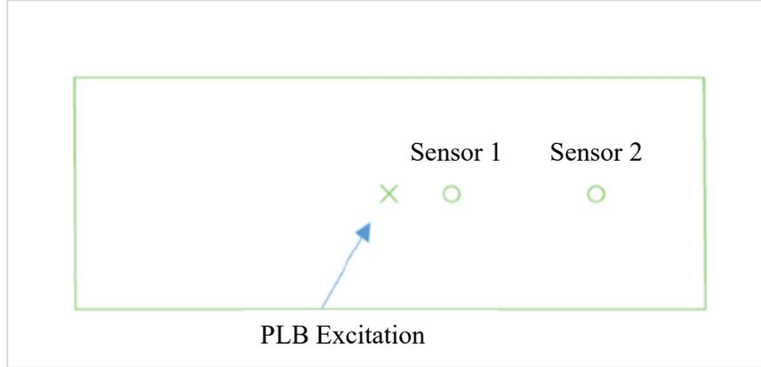
Figure 1: Sensor arrangement for wavespeed determination.
