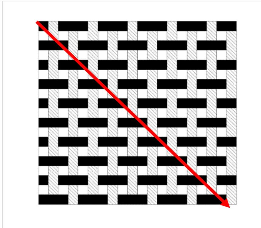
Figure 2: 45° wave propagation in a plain weave laminate.
