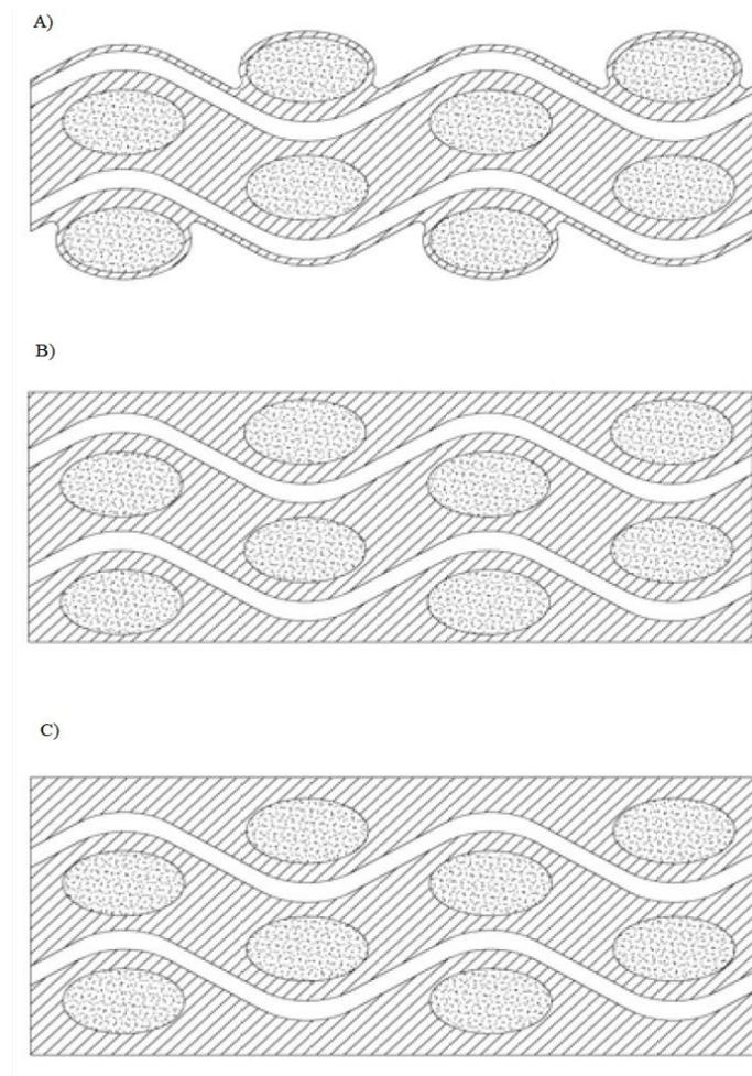
Figure 3: Cross-Sections of A) Resin Starved, B) Normal Saturation and C) Resin Rich Laminates.
