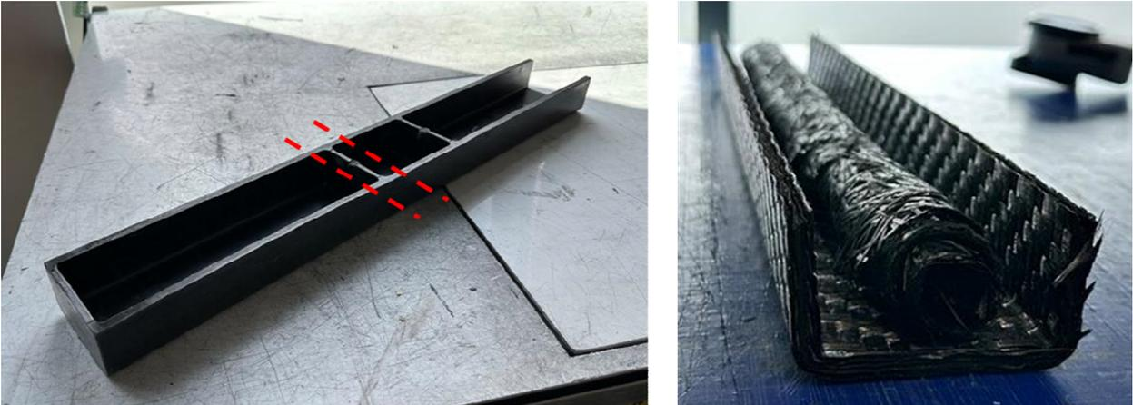
Figure 2: Left: C-channel geometry with ribs moulded using hybrid architecture material. Right: Initial material layout. The prepreg laminate was preformed into the main body of the C-channel and the SMC
