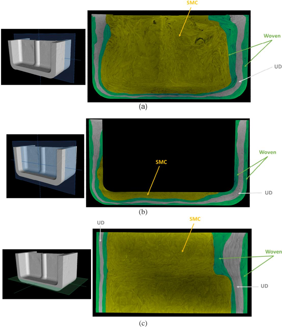
Figure 7: CT scan images for the hybrid architecture sample taken from three planes as indicated by the images on the left. The images were manually segmented to distinguish the three material phases as indicated by different colours.
