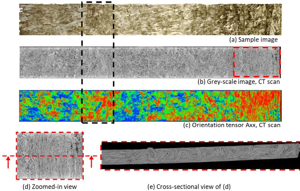
Figure 5: Comparison between (a) the image of the sample surface, (b) the grey-scale image and (c) the orientation tensor  $A_{xx}$  from the CT scan analysis for the 25mm wide sample. The black box highlights the edge of an SMC ply observed in all three images a-c. The red box indicates the edge of the plaque with (f) a zoomed-in view of the in-plane fibre architecture and (e) a cross sectional view of the out-of-plane fibre architecture.
