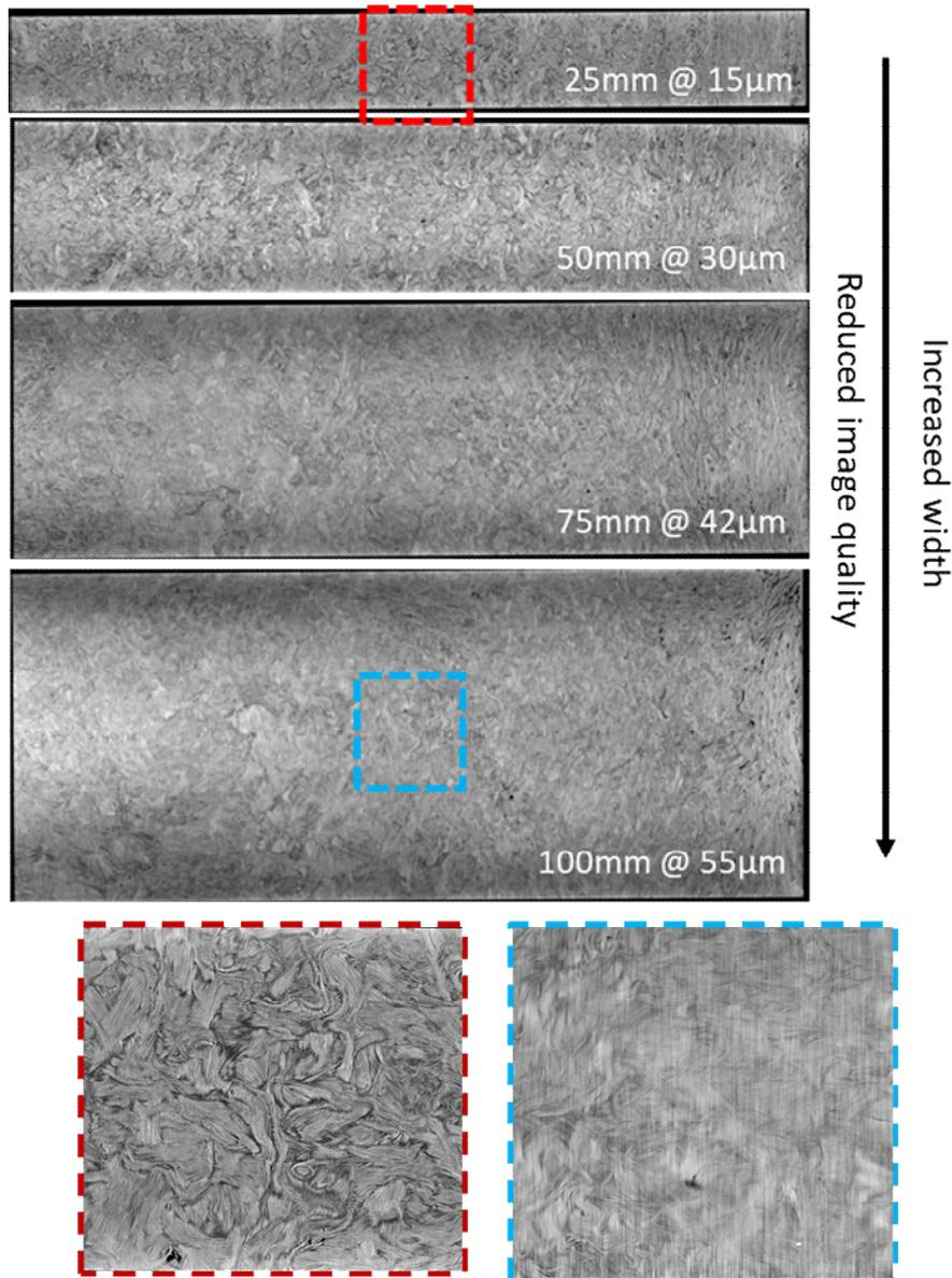
Figure 3: Comparison of grey-scale images from the CT scans for different sample widths. The red box and the blue box indicate the zoomed-in view of a 25mm x 25mm area from the 25mm sample and the 100mm sample respectively.
