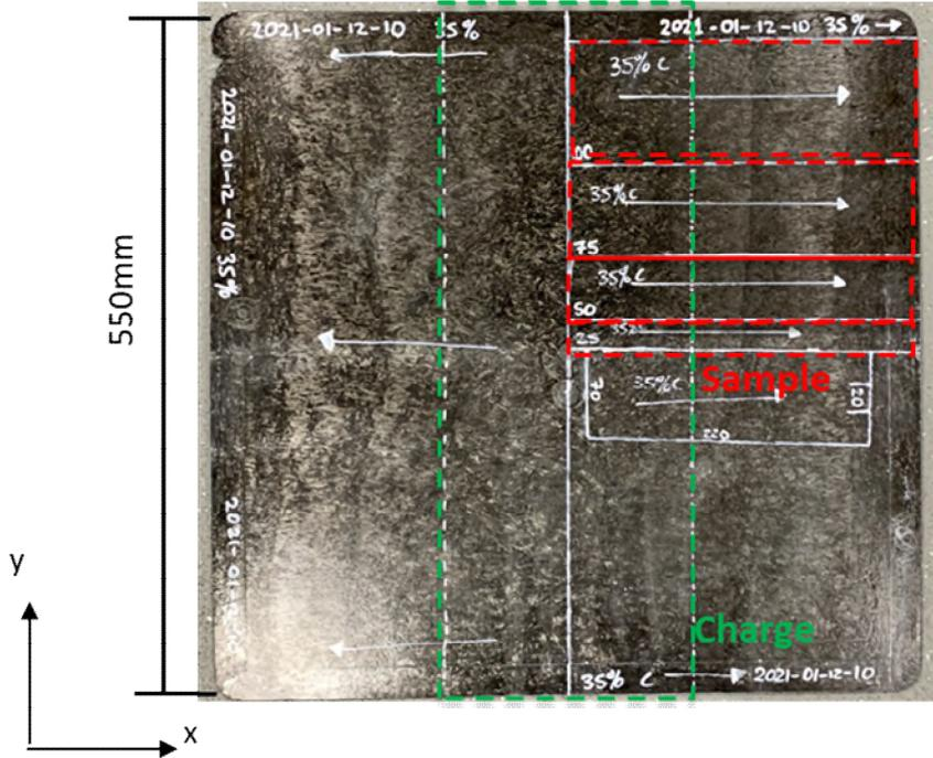
Figure 1: The flat plaque geometry with 550mm edge length and 2mm thickness. The green box indicates the initial charge location (approximately 30% centrally located), and the red boxes indicate the location of the CT samples (sample width 100mm, 75mm, 50mm and 25mm)
