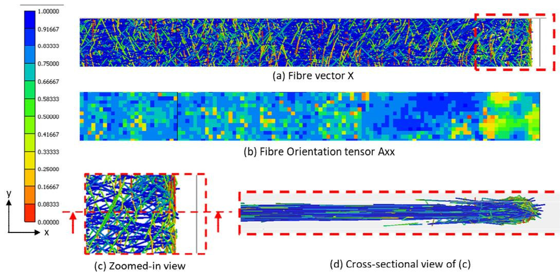
Figure 6: Fibre architecture and orientation distribution predicted for the 25mm wide sample using the DFS model in 3D TIMON. (a) Fibre vector X displayed on fibres. (b) Fibre orientation tensor Axx distribution. (c) Zoomed-in view of the fibre architecture for the region indicated by the red box in (a). (d) Cross-sectional view of (c).
