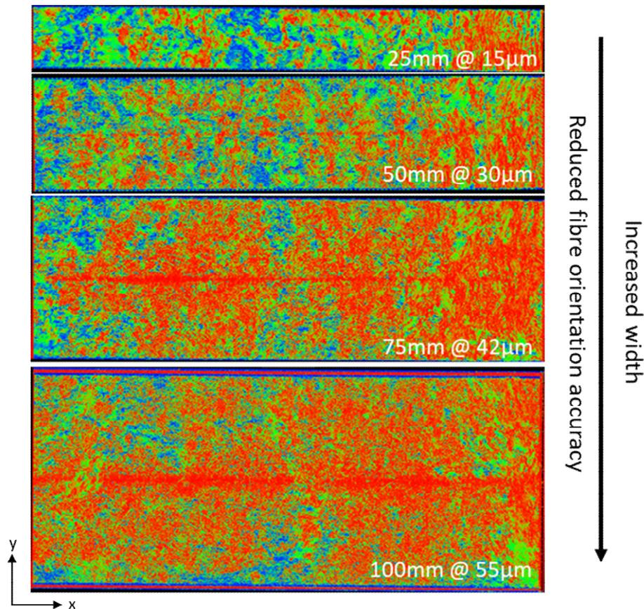
Figure 4: Comparison of fibre orientation distributions from the CT scan analysis for different sample widths. The colours indicate the fibre orientation tensor where blue represents  $A_{xx} > 0.66$ , red represents  $A_{xx} < 0.33$  and green represents the values in between.
