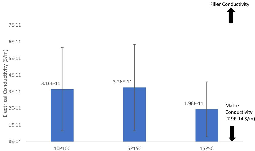
Figure 9: Variation of electrical conductivity for different filler combinations
