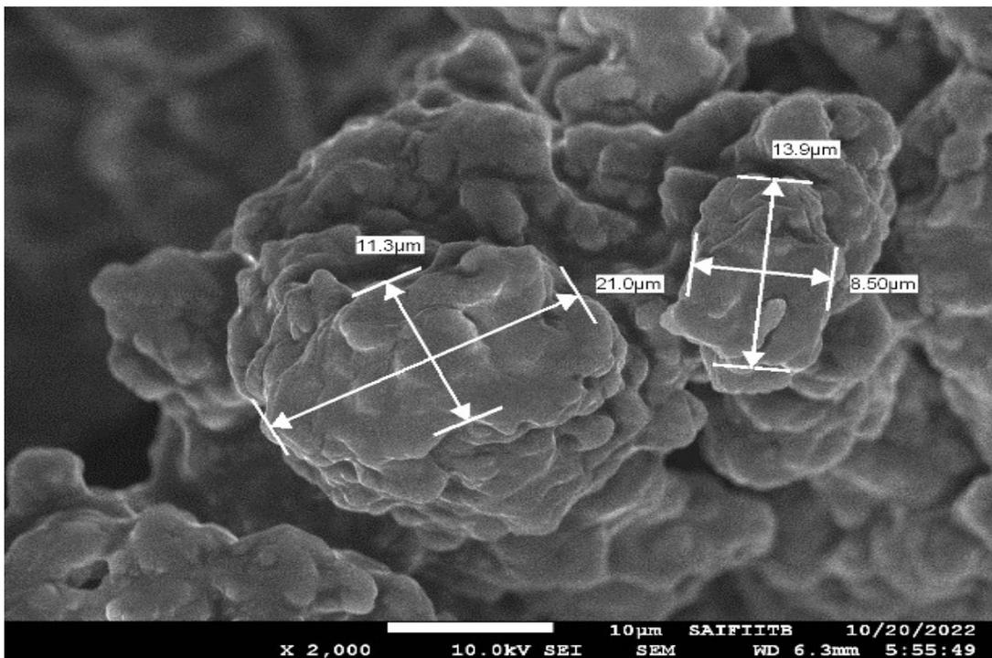
Figure 3: SEM image of Polyaniline
