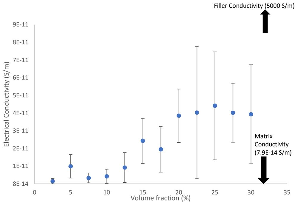
Figure 8: Variation of electrical conductivity with varying volume fraction in CB/ epoxy composites
