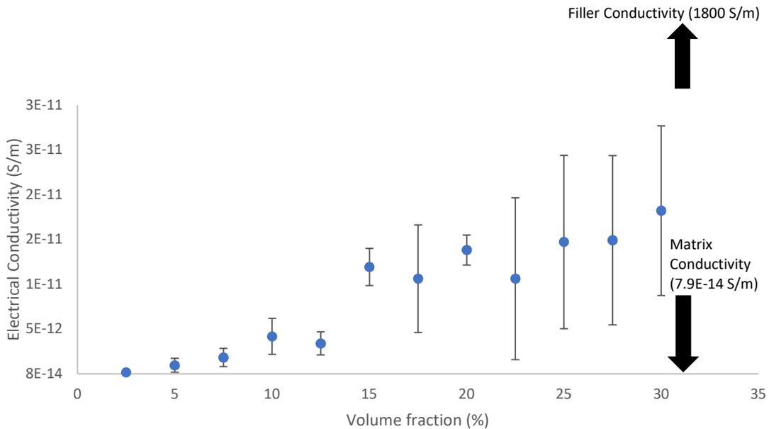
Figure 7: Variation of Electrical conductivity with varying volume fraction in PANI/ epoxy composites
