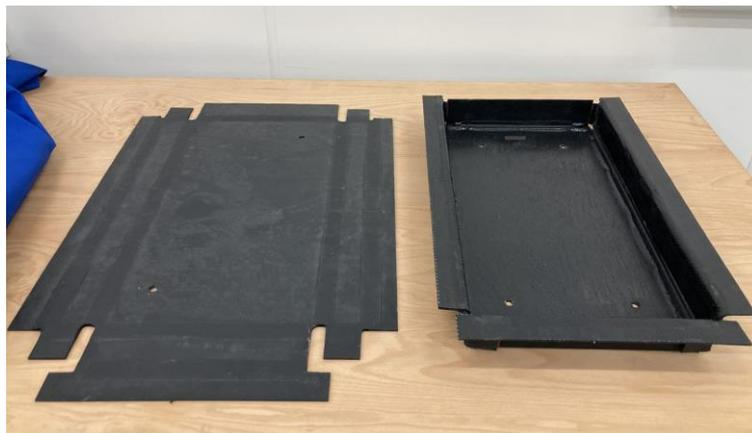
Figure 4. Full-scale 2D and 3D composite battery enclosures.
