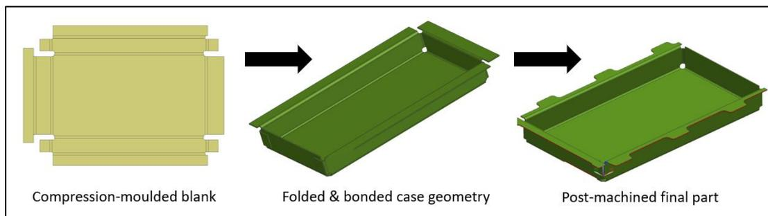
Figure 1. Example of 223<sup>TM</sup> process technology
