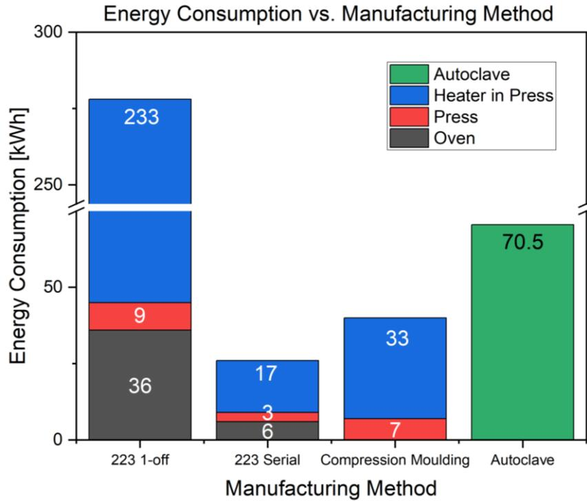
Figure 7. Total Energy Consumption of Manufacturing Methods
