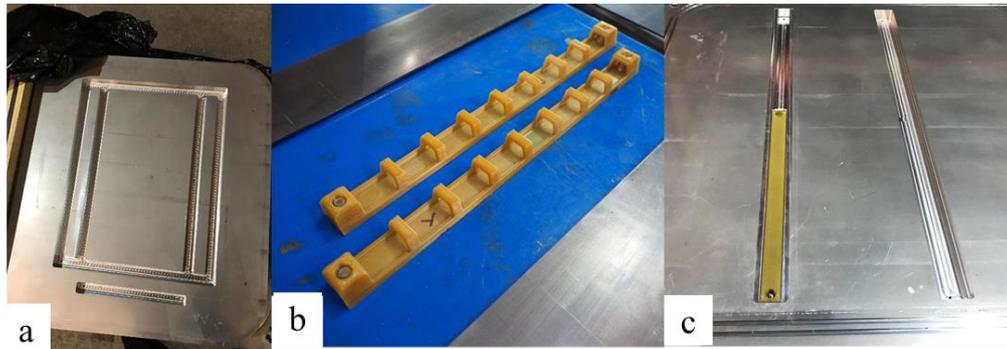
Figure 2. (a) Tooling for demonstrator (b) polymer inserts and (c) assembled coupon tooling.
