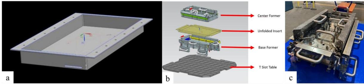
Figure 3. (a) Composite battery module case design (b) MetLase bending jig - exploded view (c) manufactured jig
