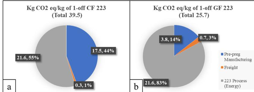
Figure 8. Kg CO<sub>2eq</sub>/kg for 1-off 223<sup>TM</sup> production with (a) CFRP and (b) GFRP.
