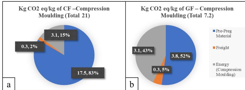
Figure 11. Kg CO<sub>2eq</sub>/kg for compression moulding with (a) CFRP and (b) GFRP
