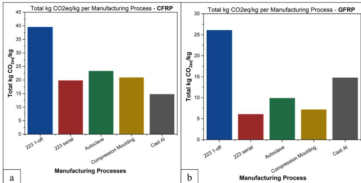
Figure 12. Total kg CO<sub>2eq</sub>/kg for all manufacturing processes with (a) CFRP and (b) GFRP.
