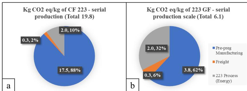
Figure 9. Kg CO<sub>2eq</sub>/kg for serial 223<sup>TM</sup> production with (a) CFRP and (b) GFRP
