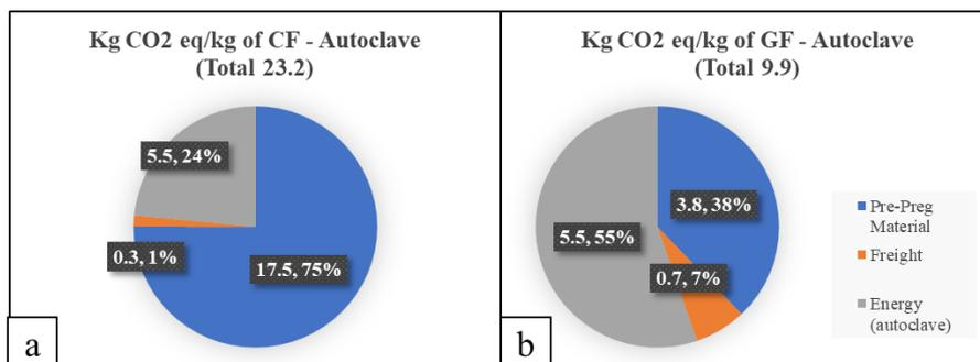
Figure 10. Kg CO<sub>2eq</sub>/kg for autoclave manufacturing with (a) CFRP and (b) GFRP
