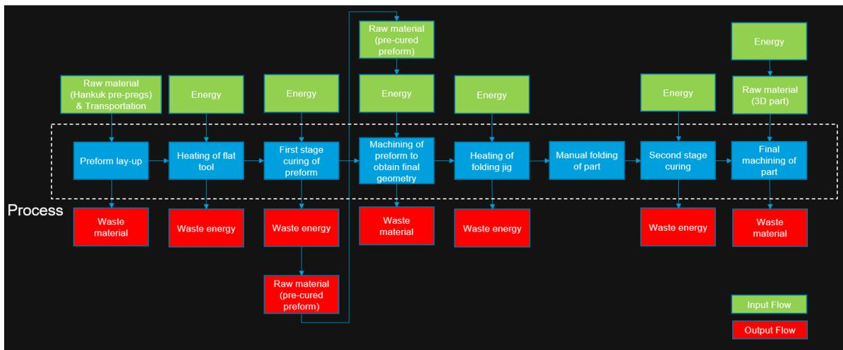
Figure 5. Process flow of 223<sup>TM</sup> manufacturing process.
