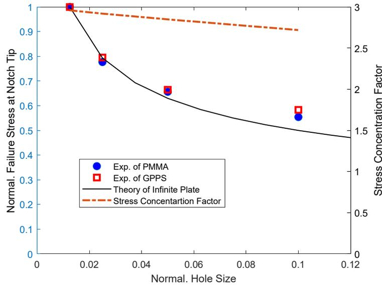
Figure 3: Plot of normalized failure stresses at the edge of the holes.
