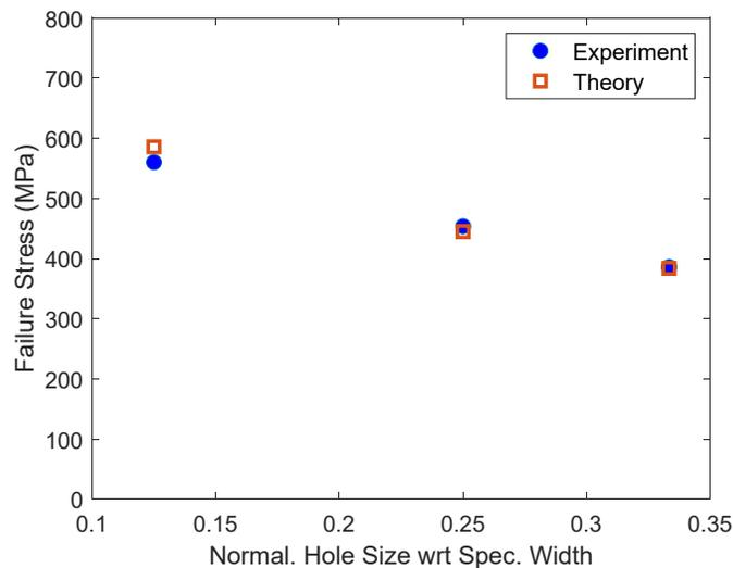
Figure 5: Comparison of failure stresses of quasi-isotropically laminated specimens.
