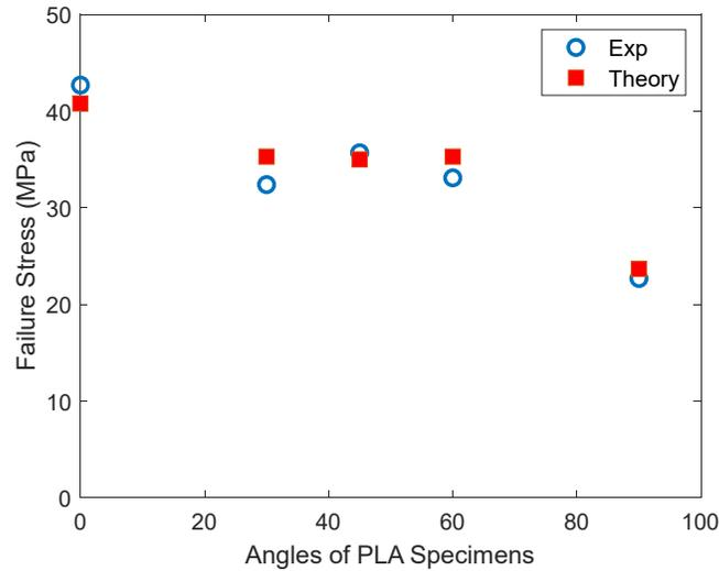
Figure 4: Comparison of failure stresses of PLA specimens with 6 mm diameter holes with different printing angles.
