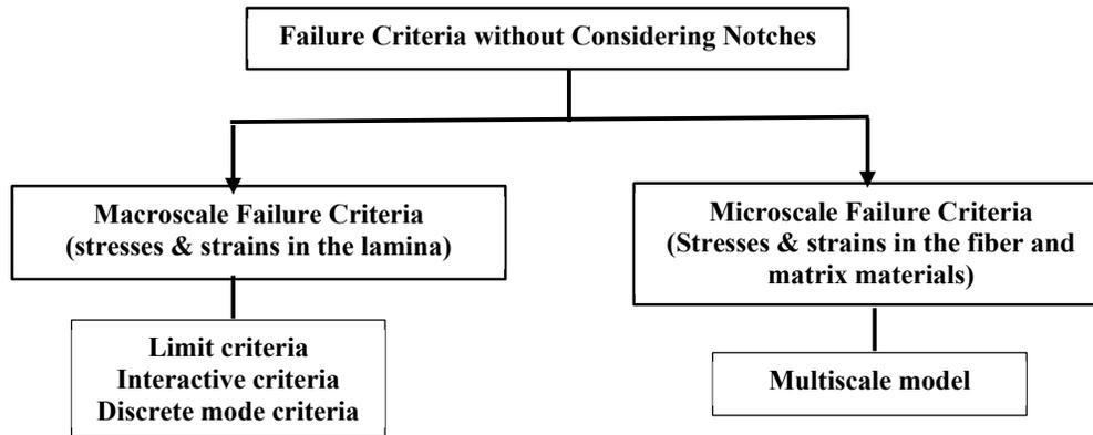
Figure 1: Classification of failure criteria without considering notches.
