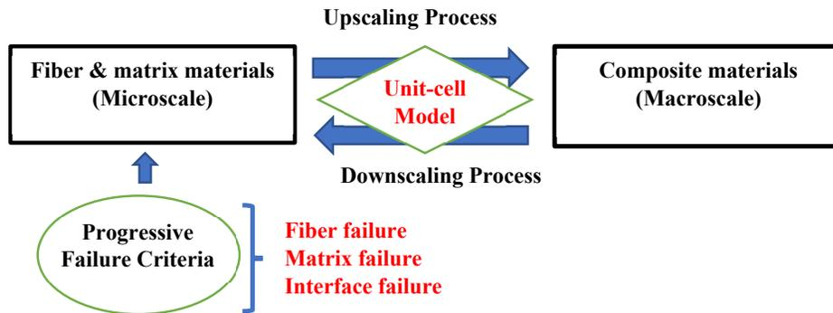
Figure 2: Microscale failure criteria based on multiscale approach.
