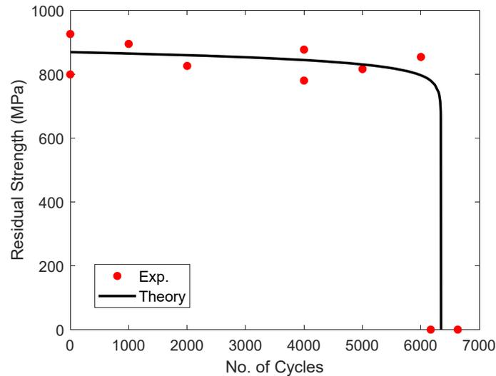
Figure 6: Comparison of residual strength of unidirectional composite subjected to cyclic loading.
