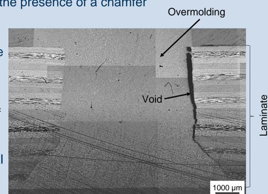
The insufficient venting causes process-induced defects leading to an early failure. Nevertheless a full pullout of the rivet-like structure from the laminate has not been observed in any test. This indicates a good adhesion to the walls of the breakthrough geometry, when intimate contact is realized.
