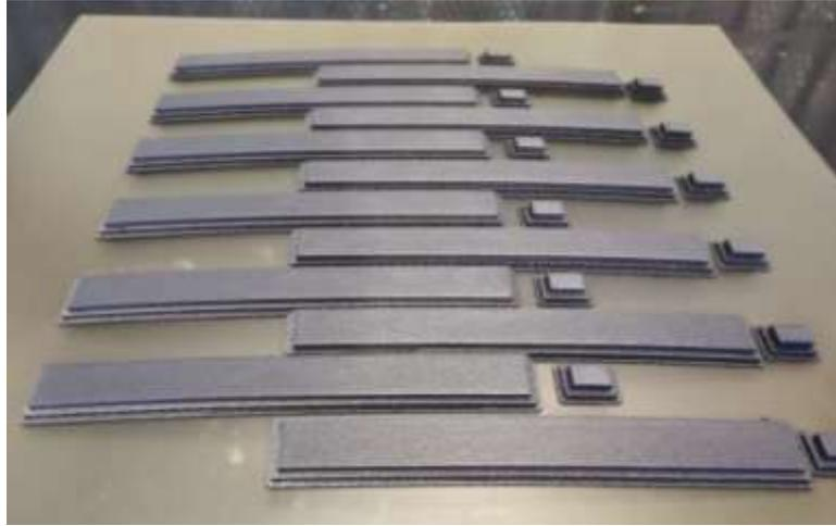
Figure 1: Printed specimens as-built before CNC machining.
