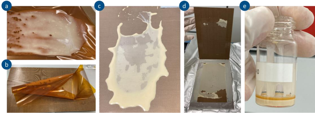
Figure 2: electrolyte samples using Araldite LY556/ XB3473 thermoset system as reinforcing agent. Samples using 40-50 vol.% (a-c), 70 vol.% (d-e) are shown after curing.
