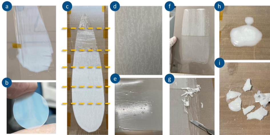
Figure 1: electrolyte samples using Araldite LY5052/ Aradur 5052 thermoset system as reinforcing agent. Samples using 20 vol.% (a,b), 40-45 vol.% (c-e), 50 vol.% (f-g), and 60 vol.% (h-i) are shown after curing.
