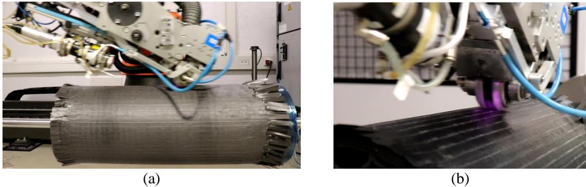
Figure 2: Split disk specimen production for the transverse tensile test placing 0° layers using the AFPisc process from the side view (a) and to the nip point (b)
