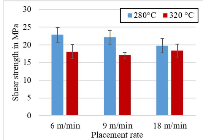
Figure 2: Valid and invalid modes of failure of the compression shear test (a) and shear strengths resulting from the AFPisc process at different placement rates and nip point temperatures (b)
