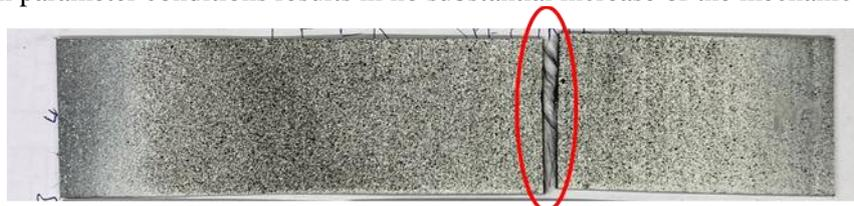
Figure 5: Failure of a transverse tensile specimens reveal dry carbon filaments
