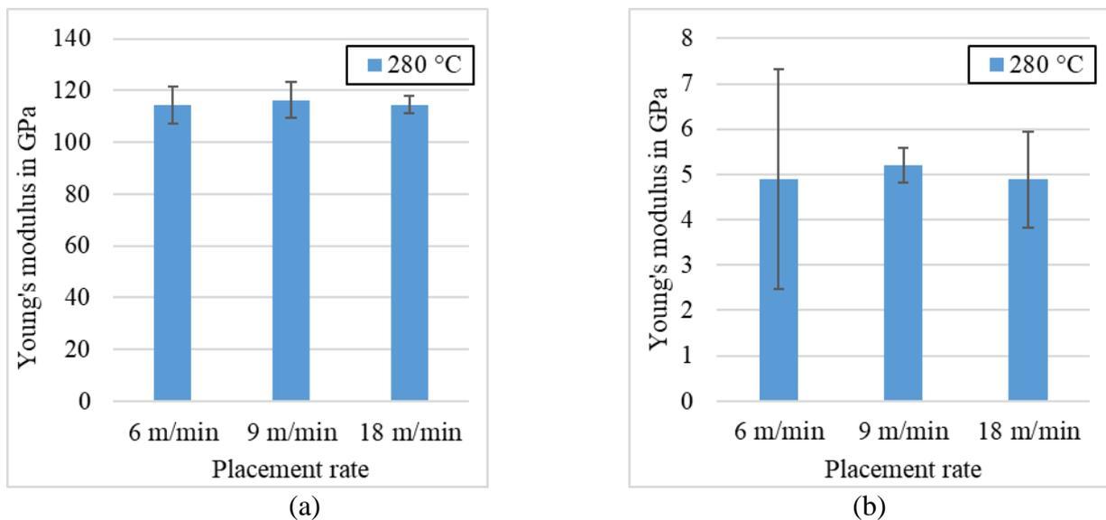
Figure 6: Young's moduli of the split disk test and different placement rates at a processing temperature of 280 °C, parallel (a) and transverse (b) to the fiber.
