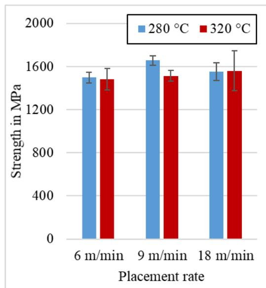
Figure 3: Tensile test results in fiber direction at different placement rates and processing temperatures at the nip point with the Young's moduli (a) and strengths (b).
