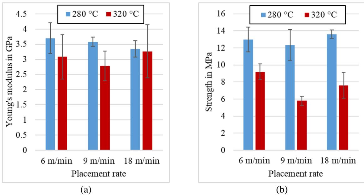
Figure 4: Tensile test results transverse to the fiber direction at different placement rates and processing temperatures at the nip point with the Young's moduli (a) and strengths (b).
