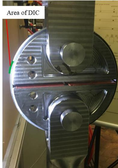
Figure 3: Split disk test fixture with marked area of digital image correlation (DIC) for the measurement of the strain
