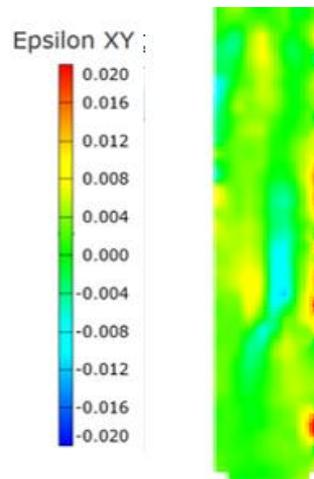
Figure 14: Characteristic H-shape at a tape discontinuity.
