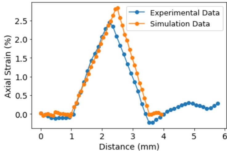
Figure 13: Axial strain by DIC and FEA versus distance from a discontinuity in fibre direction.
