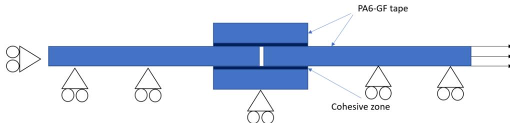
Figure 5: FEA model of the double lap shear specimens.
