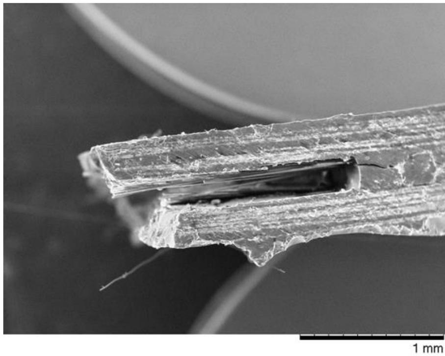
Figure 7: Remainder of double-lap shear joint after tape pull-out (x60 magnification).
