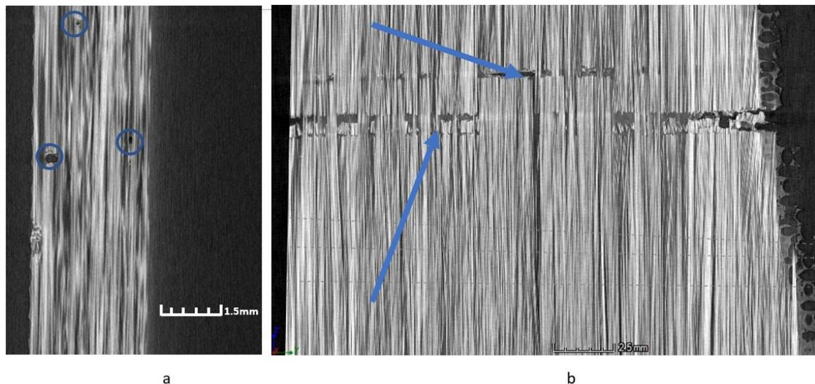
Figure 4: Geometry of the aligned brick-and-mortar showing the location of discontinuities.
