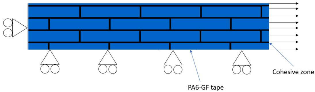
Figure 6: FEA model of the aligned brick-and-mortar specimens.
