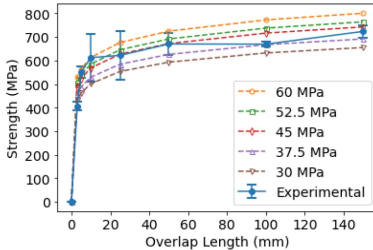
Figure 10: The effect of varying the peak traction in the cohesive zone model on FEA tensile strength predictions together with experimental data.
