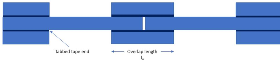
Figure 3: Double-lap shear test specimen geometry.
