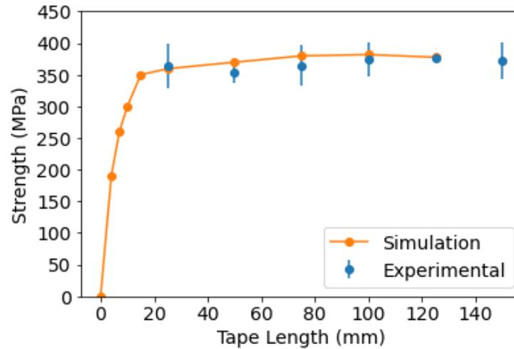
Figure 12: Influence of tape length on tensile strength of aligned discontinuous tape composites; FEA simulations versus experimental data.
