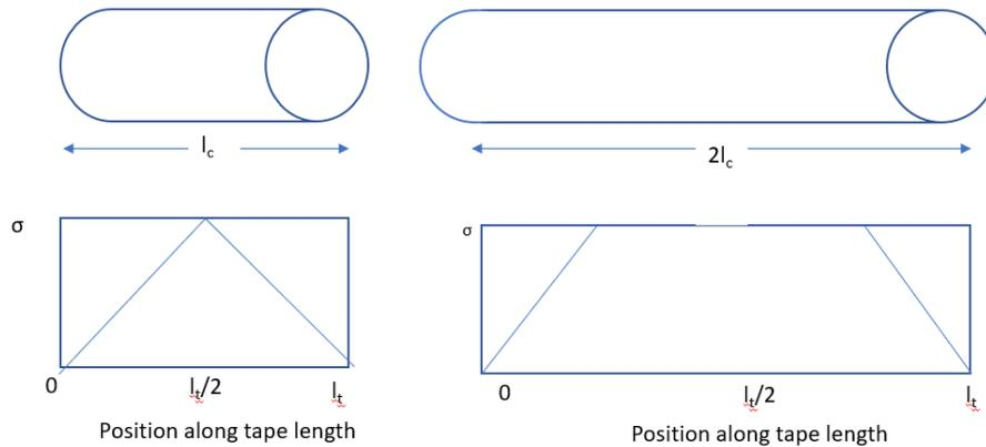
Figure 1: The analytical distribution of stress through a tape of critical length  $l_c$  (left) and twice critical length  $2l_c$  (right).
