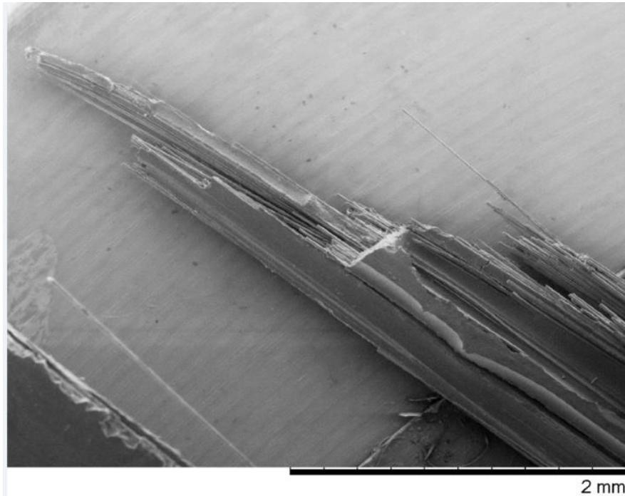
Figure 9: Broken fibres at 100 mm tape length (x50 magnification).
