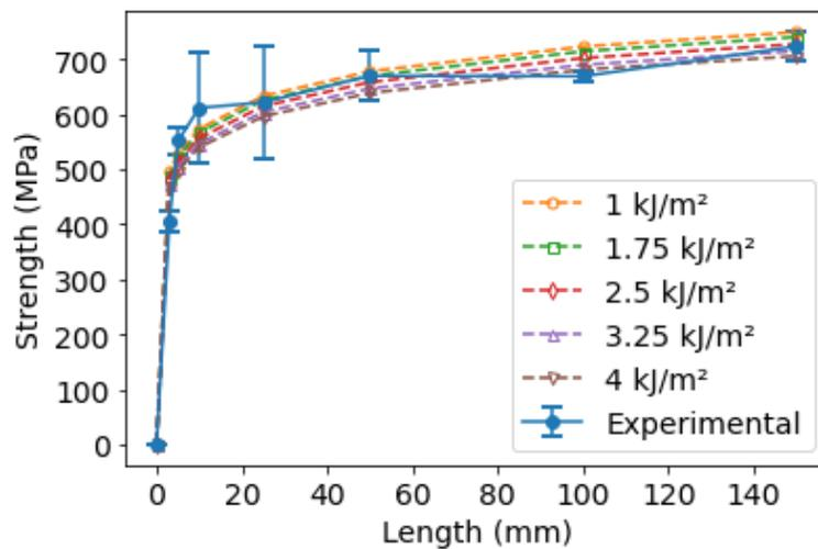
Figure 11: The effect of varying the interface fracture energy on strength for FEA simulations together with experimental data.
