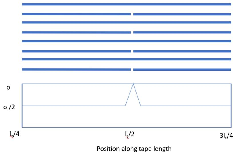
Figure 2: A schematic of the analytical effect on stress  $\sigma$  through a tape of length  $l_t$  of stacking discontinuities at location  $l_t/2$ . In this diagram, stress is only shown in the middle of the tape, which is assumed to be several times longer than the stress-transfer length.
