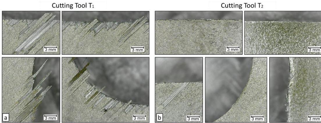
Figure 8: Machined part resultant from the third experiment: a) parts machined with cutting tool T1 and b) parts machined with cutting tool T2.
