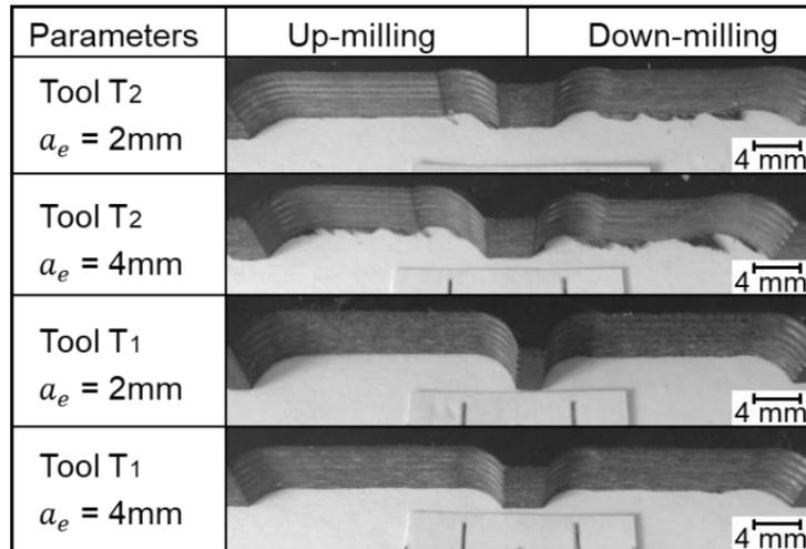
Figure 6: Machined part resultant from the second experiment.
