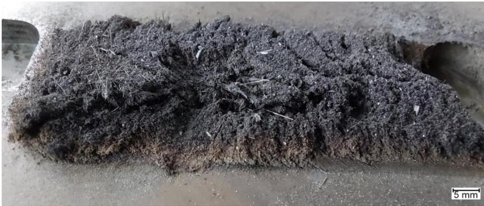
Figure 9: Burned matrix during the robot test.
