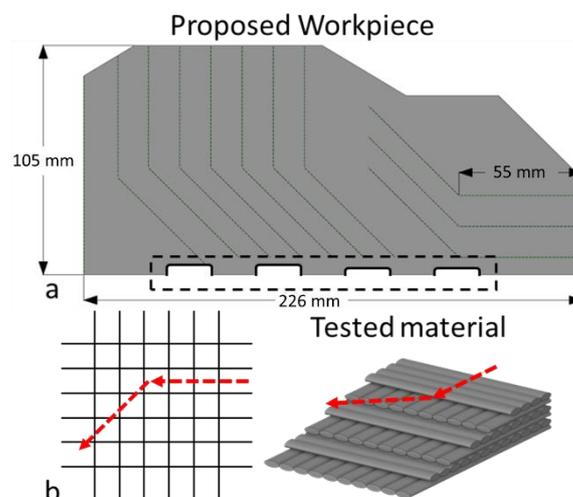
Figure 2: Proposed workpiece: a) Workpiece dimensions and cutting movements; b) Fiber alignment of the used material and the executed movements during the test.
