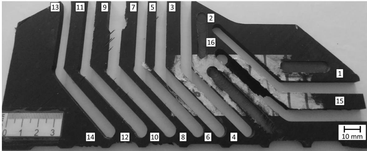
Figure 4: Machined part resultant from the first experiment.
