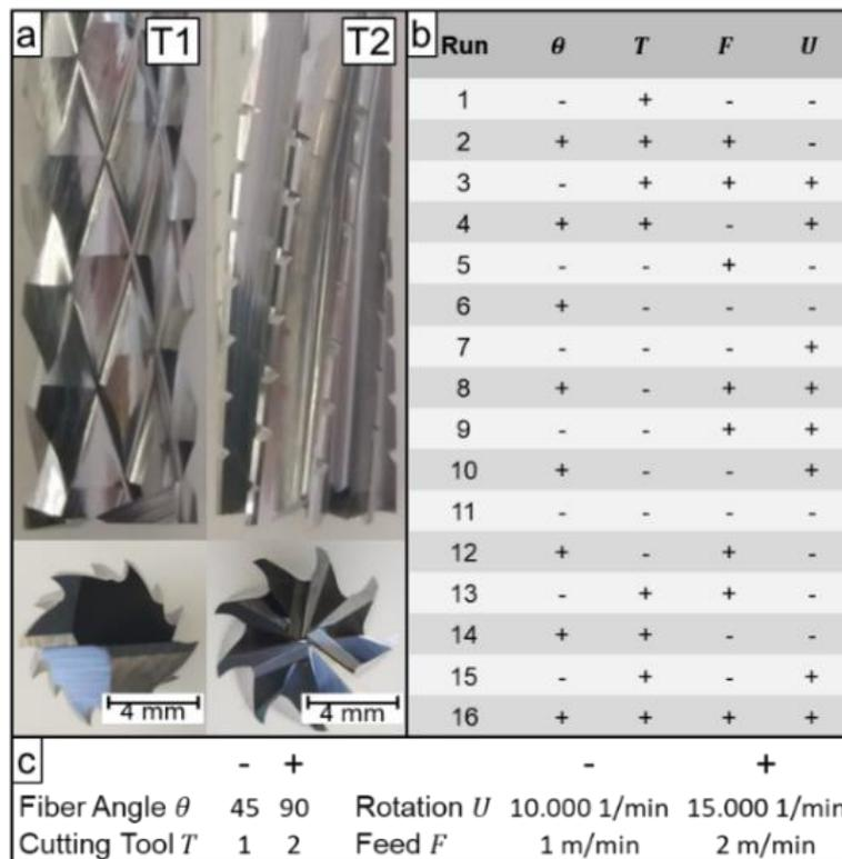
Figure 1: Experimental design: a) Tools used; b) Factors analyzed and c) the values for each factor.
