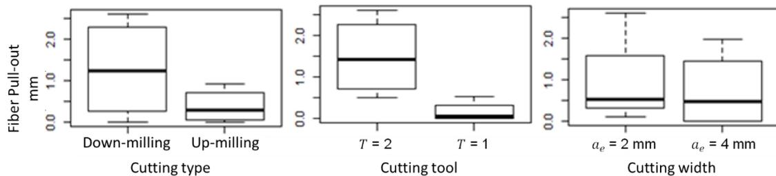
Figure 7: Box plot diagrams of the results for the tested parameters.
