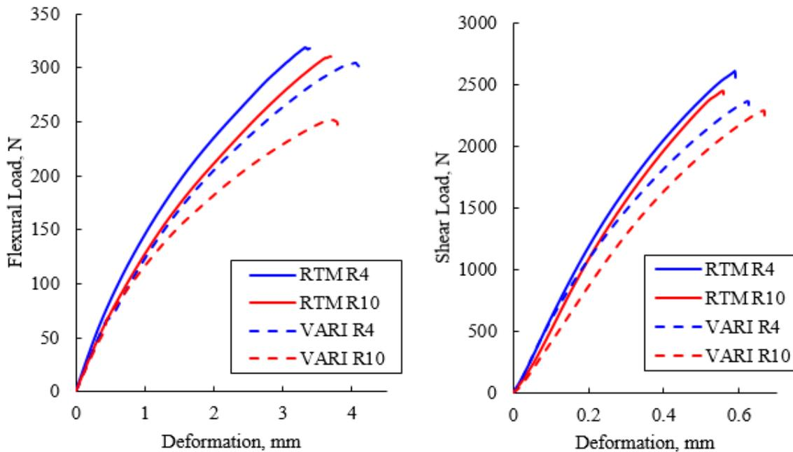
Figure 5: Load-deformation curve under flexural and shear loading
