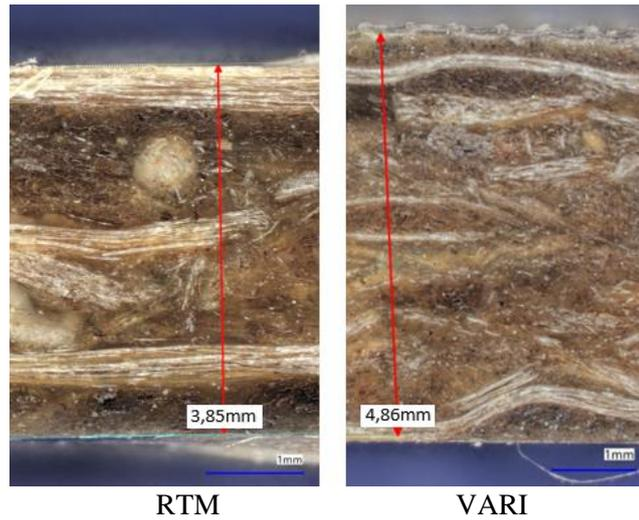
Figure 4: Sandwich composite panels thickness variation of RTM and VARI process
