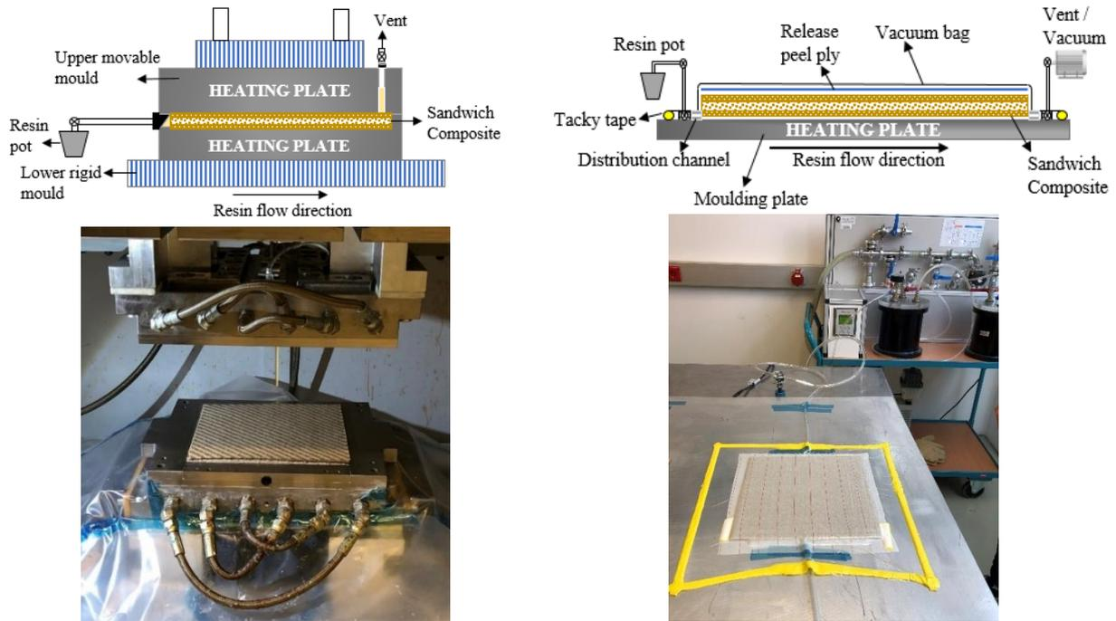
Figure 1: Schematic representation of RTM and VARI
