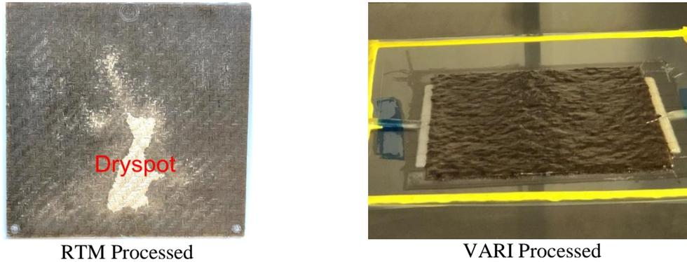
Figure 2: Challenges in manufacturing sandwich composite panel in RTM and VARI
