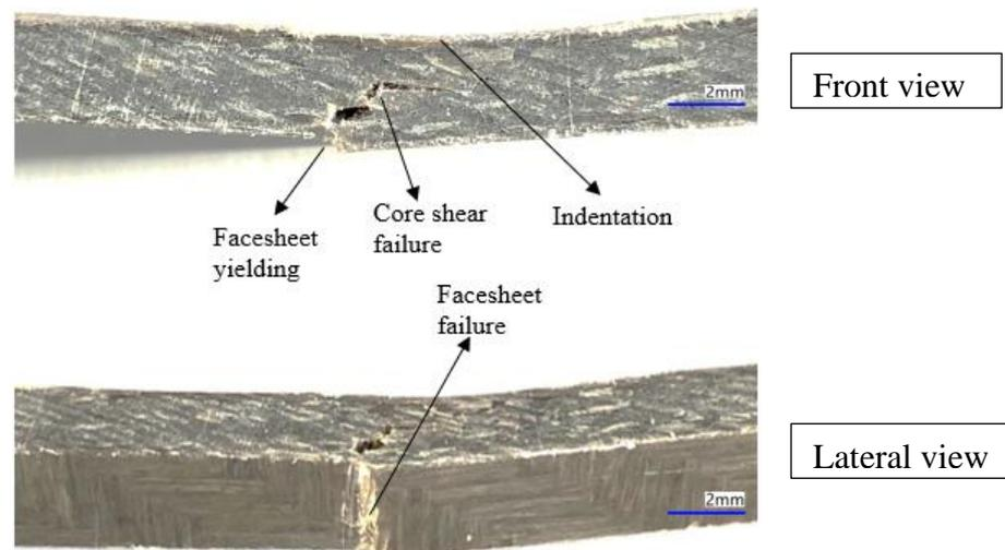
Figure 6: Failure types in flexural and shear loading. (Top) Front view and (Bottom) Lateral view of sandwich composite panels
