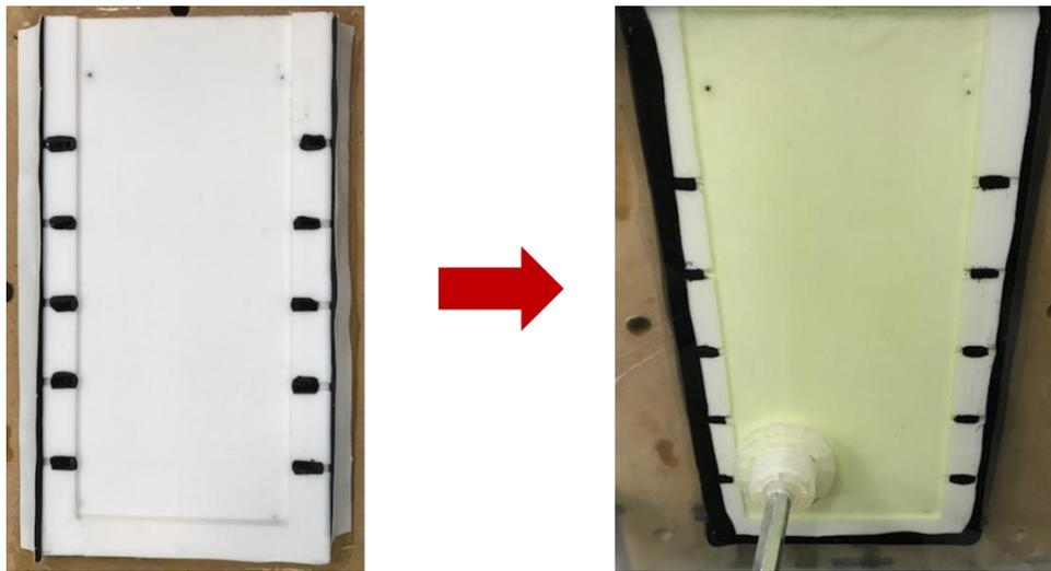
Figure 1: Mould setup utilized for curing Elium<sup>®</sup> plaques containing embedded single carbon fibres. The channels can be observed by the placement of the sealant tape.
