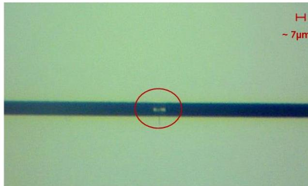
Figure 4: Image showing a fibre fragmentation within a carbon fibre whilst under 250x magnification.
