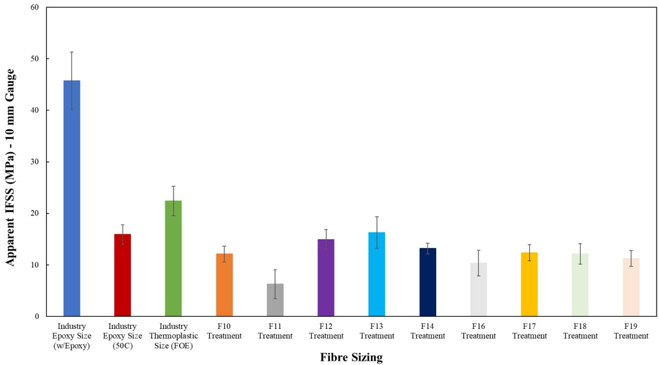
Figure 5: Comparative plot showing apparent IFSS values measured for different coated fibres embedded within epoxy or Elium® (10 mm gauge).
