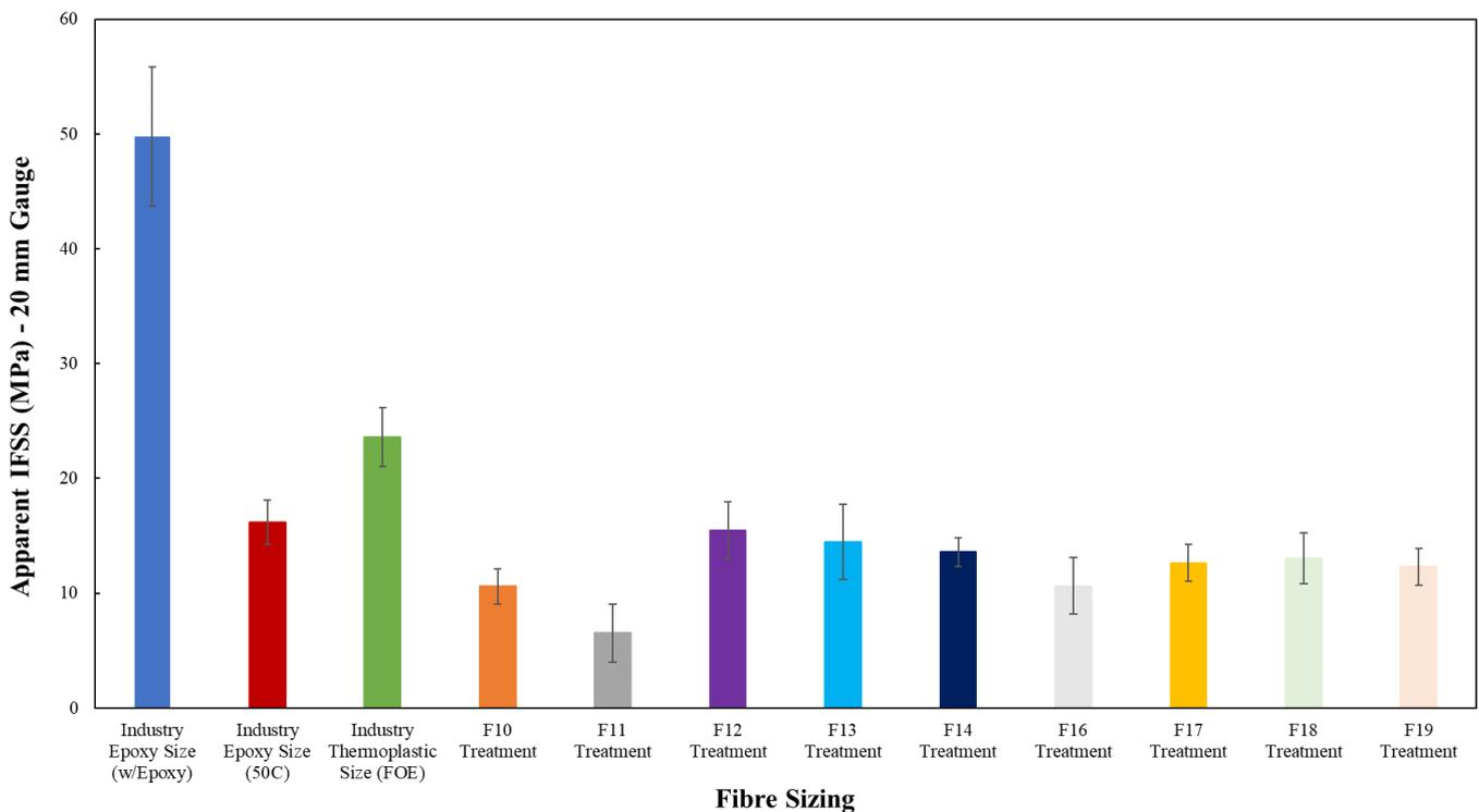
Figure 6: Comparative plot showing apparent IFSS values measured for different coated fibres embedded within epoxy or Elium® (20 mm gauge).
