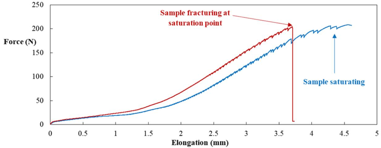
Figure 3: Force-Elongation plot for two fragmentation samples, with one having fractured at the saturation point.
