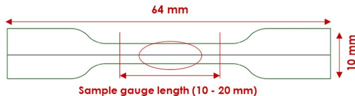
Figure 2: Geometry of SFFT samples with a thickness of 2 mm.
