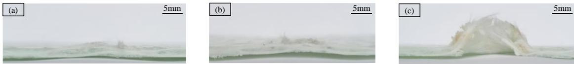
Figure 10. Side view of  $[G^{60}]_2$  laminates under certain LVI energies, (a) 15 J, (b) 30 J, (c) 60 J
