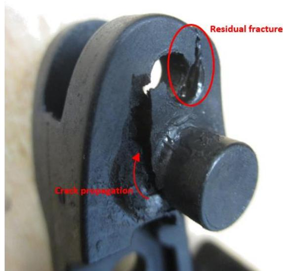
Figure 11: Fracture after cyclic loading.
