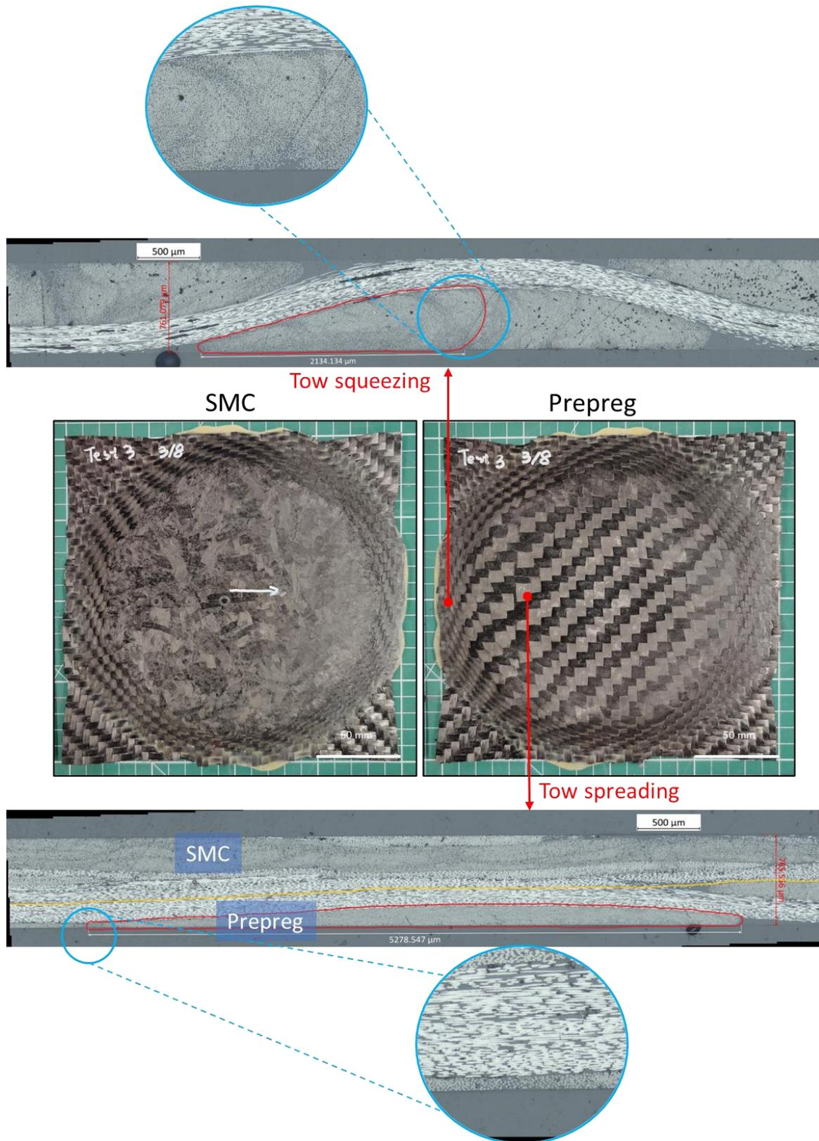
Figure 8: Hybrid-architecture specimen after the compaction test and micrographs of its cross-section.
