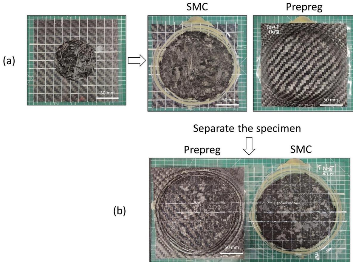
Figure 9: (a) Hybrid-architecture specimen with BOPP films inserted between prepreg and MSC and (b) the interface of two materials
