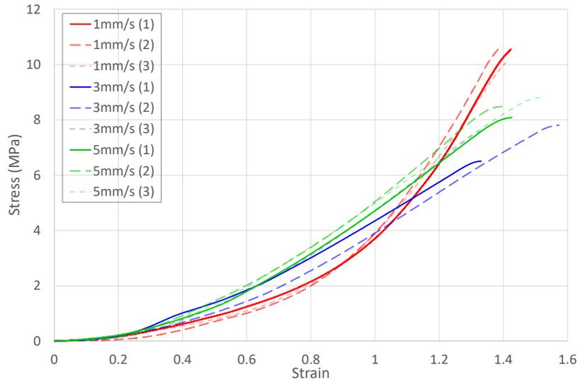
Figure 4: Compressive stress-strain curves for SMC-only specimens tested at different closing speeds.
