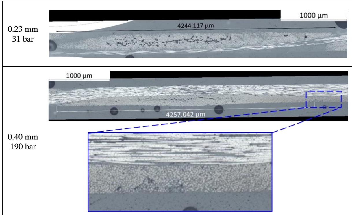
Figure 7: Micrographs of cross-sections of prepreg-only specimens at different plate displacement/pressure levels.
