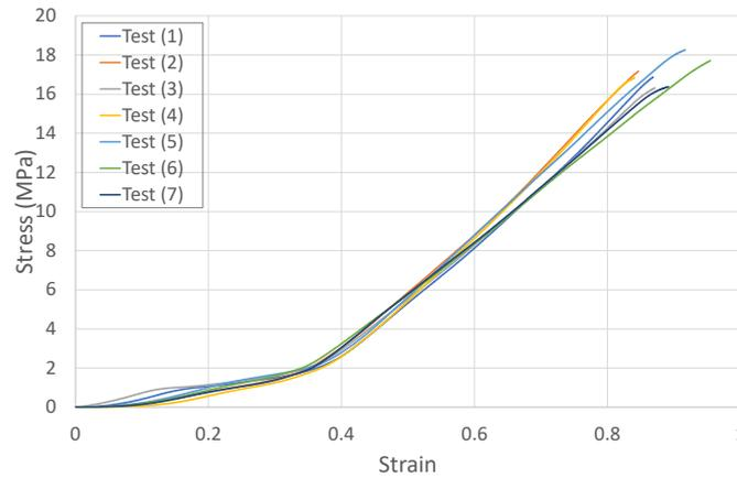
Figure 6: Compressive stress-strain curves for prepreg-only specimens
