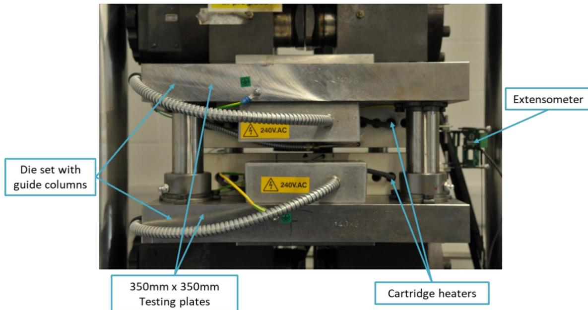
Figure 1: Squeeze flow rig on a servo-hydraulic testing machine.
