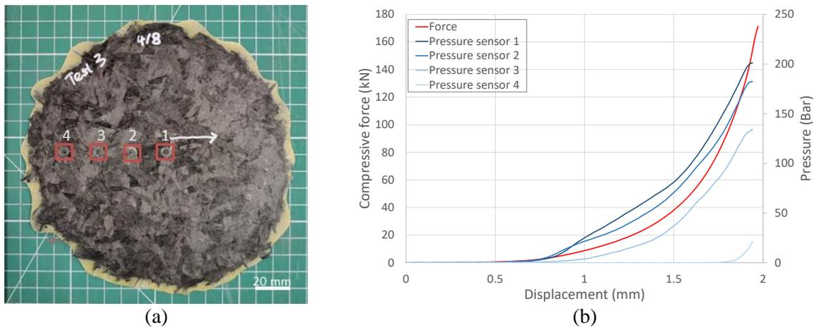
Figure 3: (a) SMC-only (configuration 1) specimen after the test and (b) compressive force and pressure – displacement curves for an SMC-only specimen tested at 100°C and 5 mm/s.
