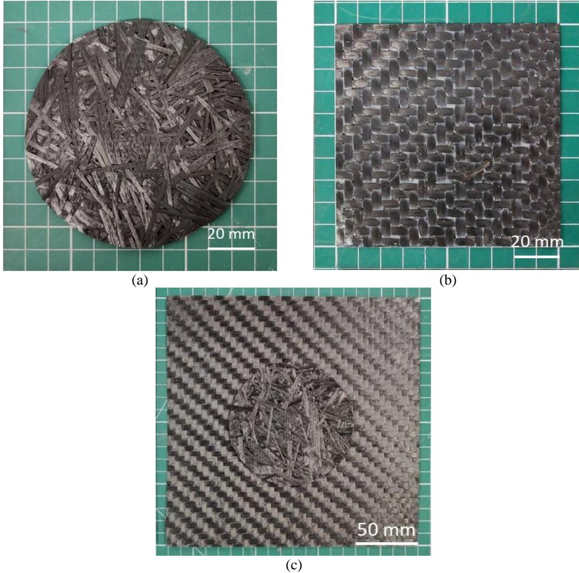
Figure 2: Untested specimens: (a) configuration 1 (SMC only), (b) configuration 2 (prepreg only) and (c) configuration 3 (hybrid architecture).
