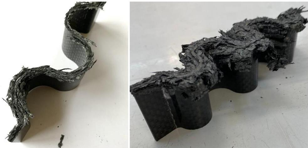
Figure 10: Crushed morphologies of the sinusoidal structures; 3 curvatures (left), 5 curvatures (right).
