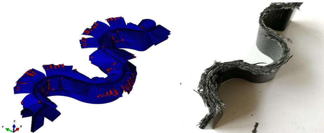
Figure 12: Crushed morphology of sinusoidal structure with 3 curvature; FE model (left) (red elements are damaged), experimental (right).
