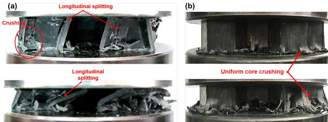
Figure 4. (a) failure in five-cell CF/epoxy honeycombs and (b) failure in CF/Elium<sup>®</sup> honeycombs.
