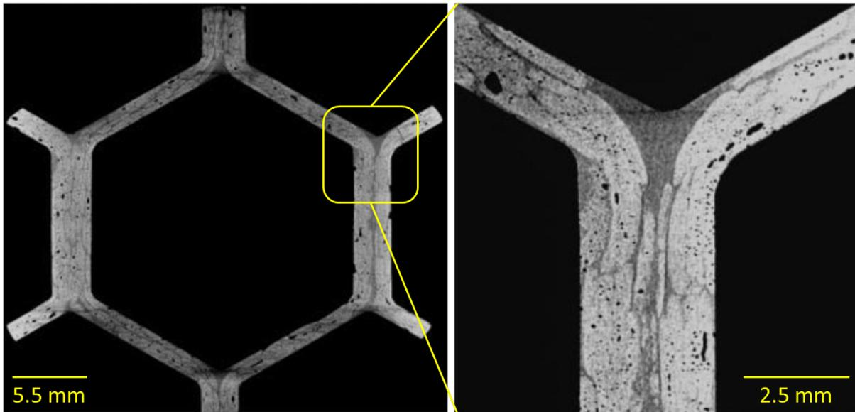
Figure 2. XCT cross-sectional images of the CFRP/epoxy honeycombs having four carbon fiber layers.
