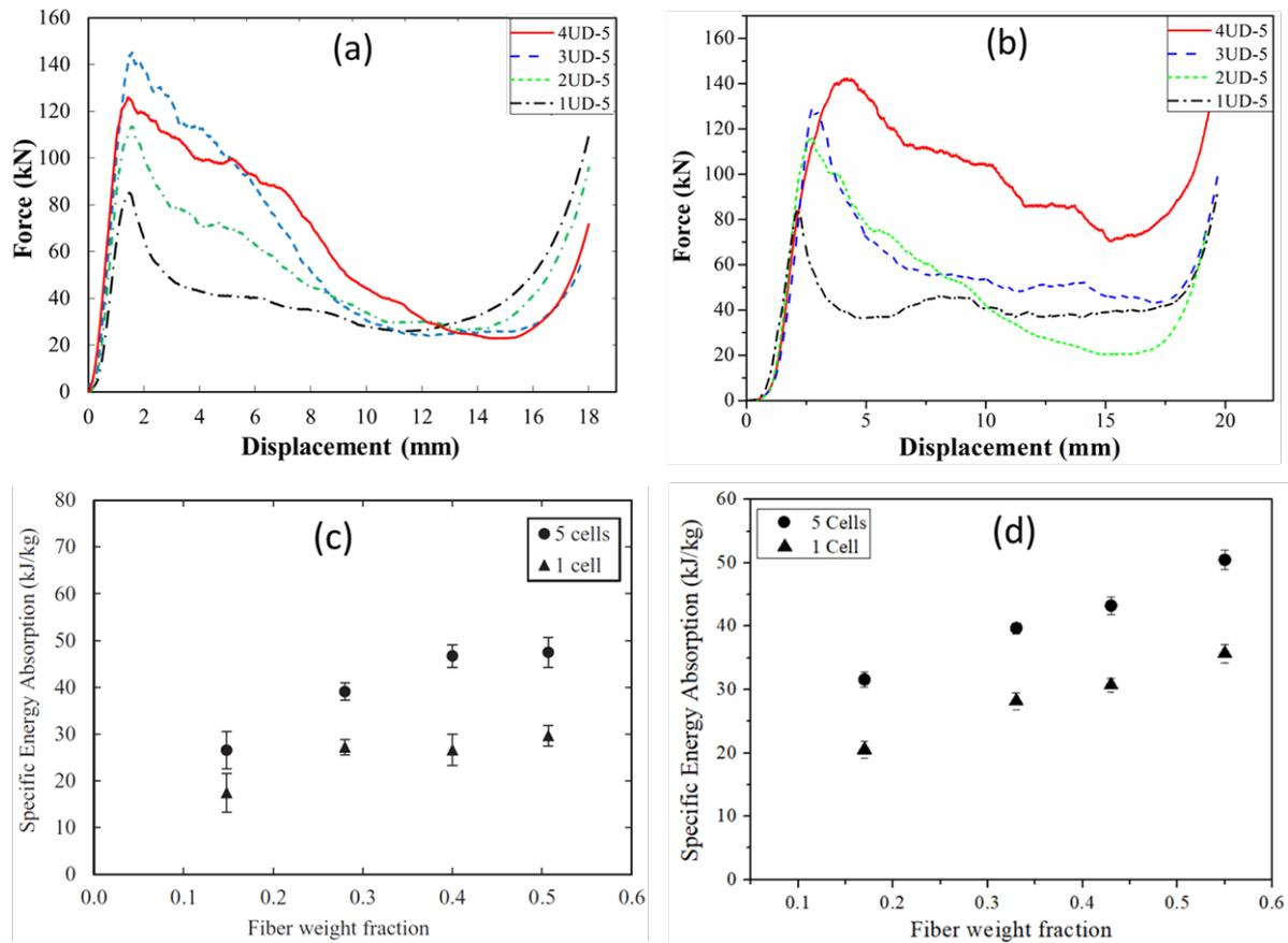
Figure 3. Compression test results (a) load-displacement curves for CF/epoxy honeycombs, (b) load-displacement curves for CF/Elium<sup>®</sup> honeycombs, (c) SEA for CF/epoxy honeycombs and (d) SEA for CF/Elium<sup>®</sup> honeycombs.
