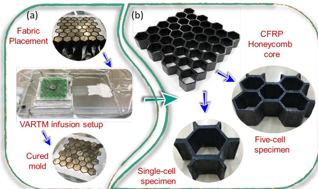
Figure 1: Manufacturing of composite honeycombs (a) mold preparation and infusion setup and (b) final composite specimens.
