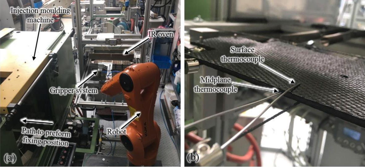
Fig. 2: Overmoulding setup for ribbed plate component (a), showing positioning of thermocouples for in-situ temperature measurements.
