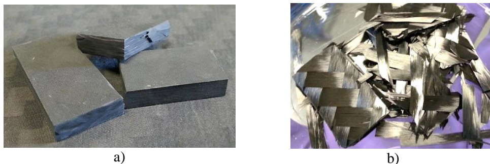
Figure 3: a) Samples of T700 fibre reinforced RTM6 epoxy; b) Fibres recovered after solvolysis (experiment #17 in Table 2).
