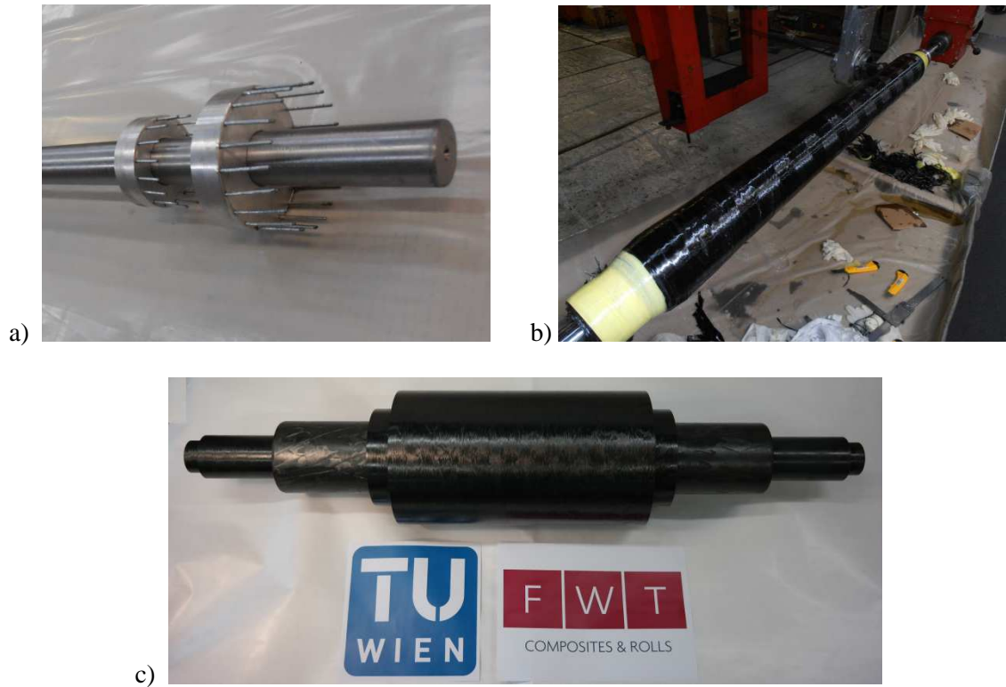
Figure 8: CFRP hollow shaft: (a) mandrel with symmetric mounted winding-pins; (b) winding of the hollow shaft; (c) finished machined shaft.
