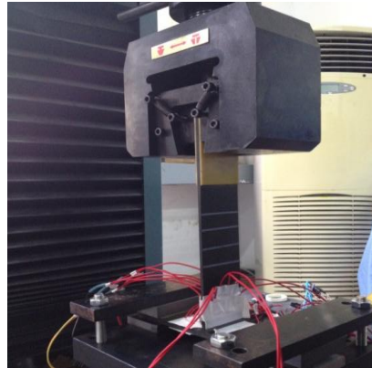
Figure 2: Test setup of pull-off tests
