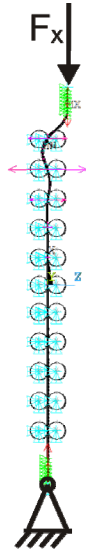
Fig. 4. First buckling mode of the supported standard specimen at a critical compressive force of F_x=4.5 kN
