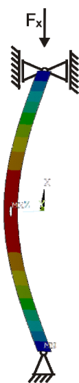
Fig. 2. First buckling mode of the unsupported standard specimen at a critical compressive force of F_x=40.5 N
