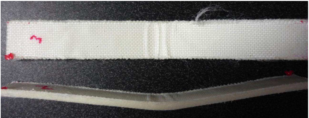
Figure 7. Impact damage of a HMPP 150 specimen.
