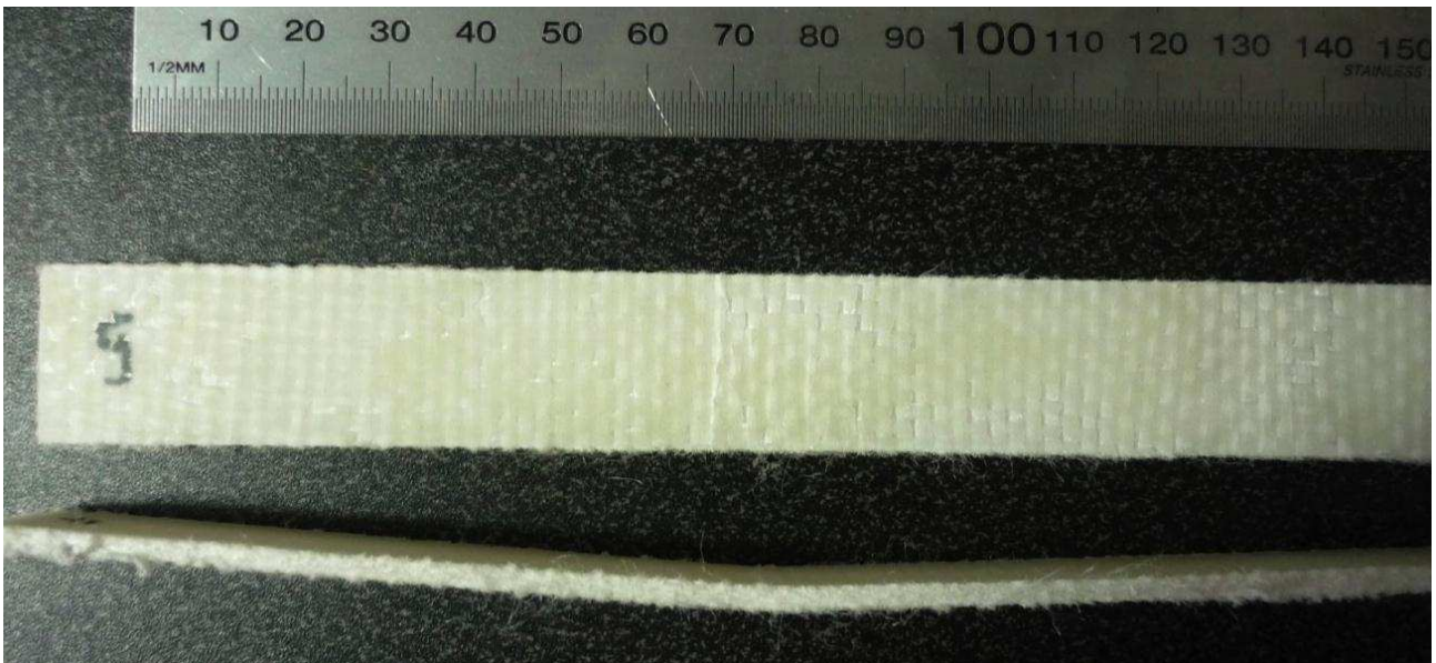
Figure 8. Impact damage of a HMPP 410 specimen.
