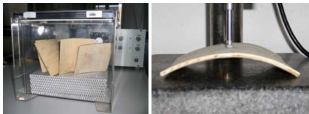
Fig. 8. Conditioning of spruce laminate in climatic case (left) and deformation with moisture saturation (right).
