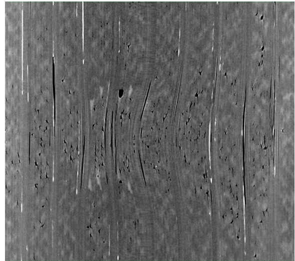
Fig. 3. Two-dimensional slice of a CT volume for a thick Carbon/Epoxy laminate with ply-waviness and porosity.
