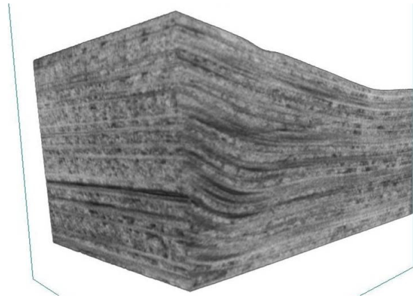
Fig. 2. A CT volume slice shows wrinkles and voids in a Glass/Epoxy laminate structural detail.
