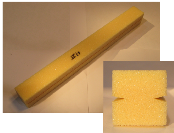
Fig. 4. An example of polymeric H100 foam specimen and cross section with notches.
