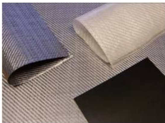
Figure 3. Example of sheet and fabric forms of self reinforced polypropylene
