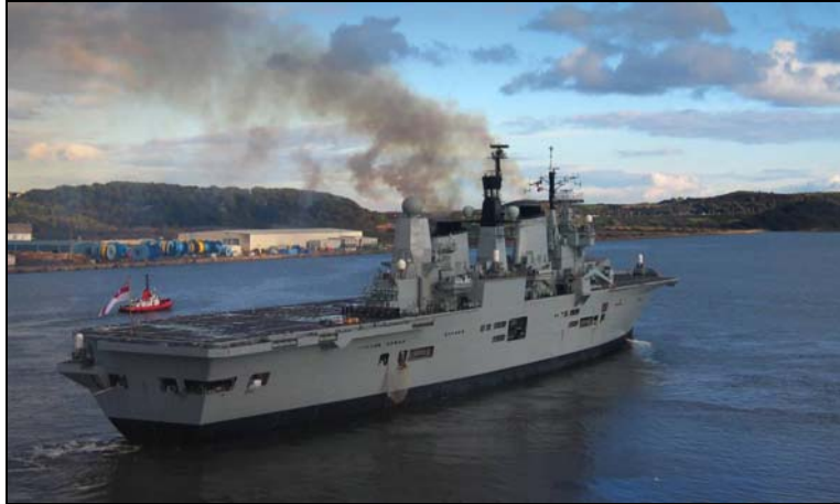
Figure 8: HMS Ark Royal reconfigured with the Advanced Technology Mast
