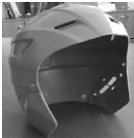
Figure 2. Ski helmet prototype made by injection moulding of a toughened r-PET.
